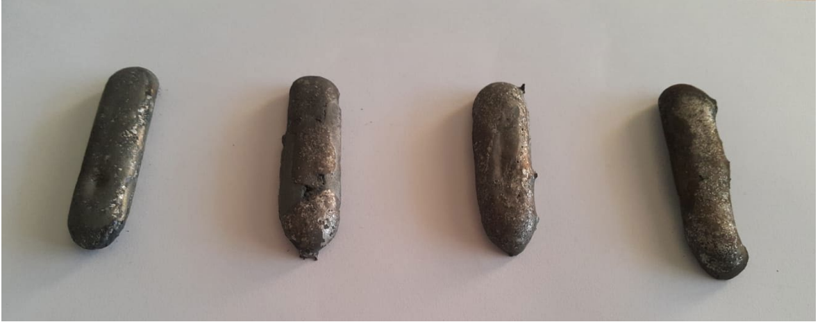
Şekil 2.4. Ark Eritme ile üretilen numuneler (Soldan 1. numune \text{Cr}_{20}\text{Mn}_{20}\text{Fe}_{20}\text{Co}_{20}\text{Ni}_{20} , 2. numune \text{Cr}_{20}\text{Mn}_{17}\text{Fe}_{20}\text{Co}_{20}\text{Ni}_{20}\text{WC}_3 , 3. numune \text{Cr}_{20}\text{Mn}_{15}\text{Fe}_{20}\text{Co}_{20}\text{Ni}_{20}\text{WC}_5 , 4. numune \text{Cr}_{20}\text{Mn}_{10}\text{Fe}_{20}\text{Co}_{20}\text{Ni}_{20}\text{WC}_{10} )
