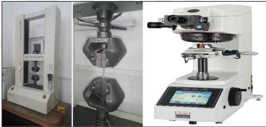
Figure 5.5. SHIMADZU tensile test and hardness measurement device [107].
