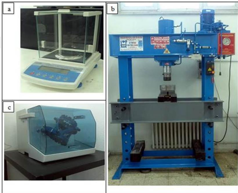
Figure 5.2. Images of a) Precision balance, b) Hydraulic press machine, and c) Powder mixing device used in experimental studies.
