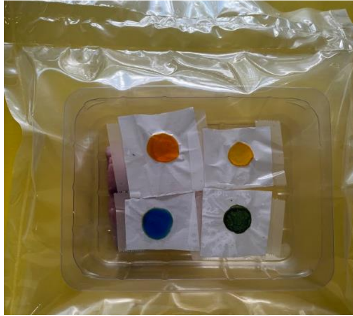
Figure 3.3. Freshness indicators set-up in the package for the food application.
