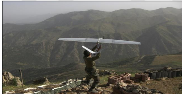
Figure 1.17 Bayraktar-Mini UAV, utilized in Internal Security Operation [24]
