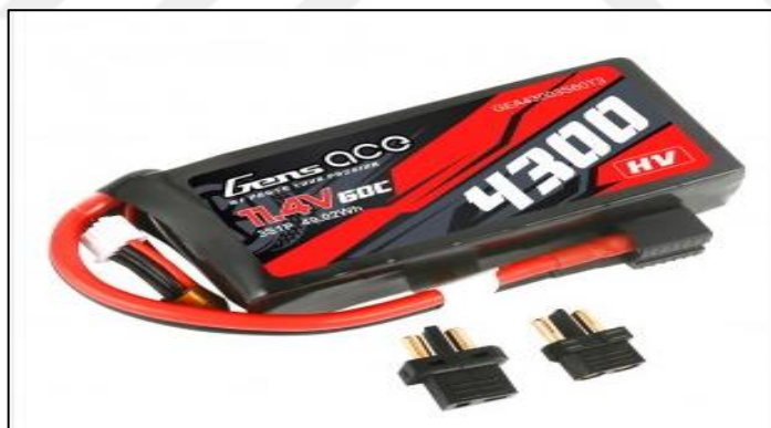
Figure 3.5 Gens Ace 4300mAh 3S1P 11.4V 60C LiHV Battery [52]
