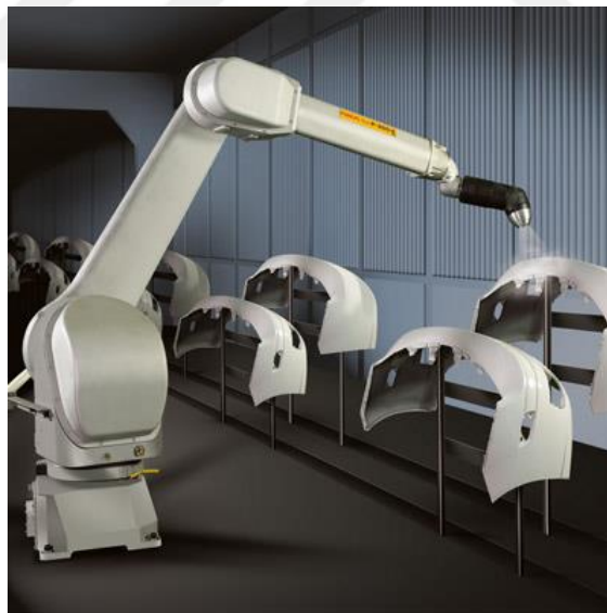
Figure 3.7: Automated Painting Executed by Stationary Robot [55].
