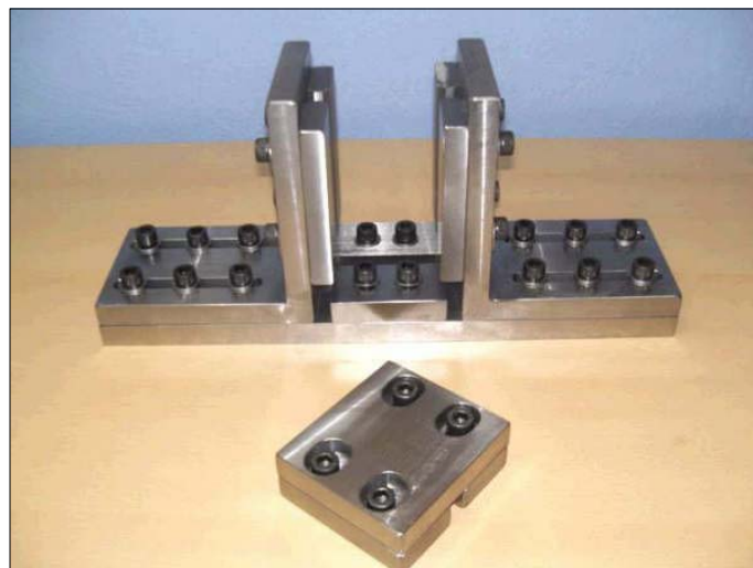
Figure 5.51 Compression after impact (CAI) test fixture
