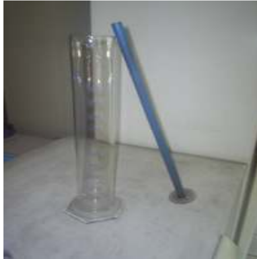
Figure 3.7. Graduated cylinder and plunger used in the laboratory tests.
