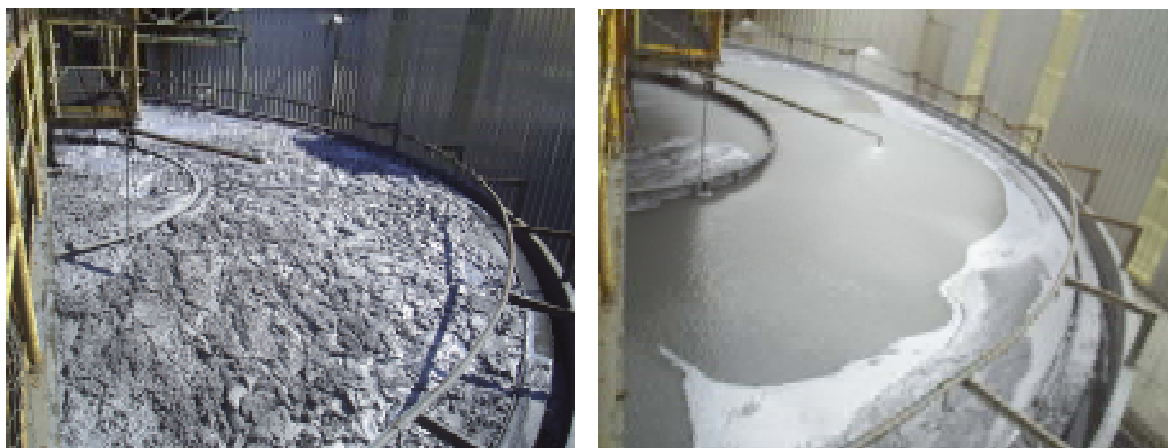
Figure 4.35. The view of Zn thickener before and after water spray application
