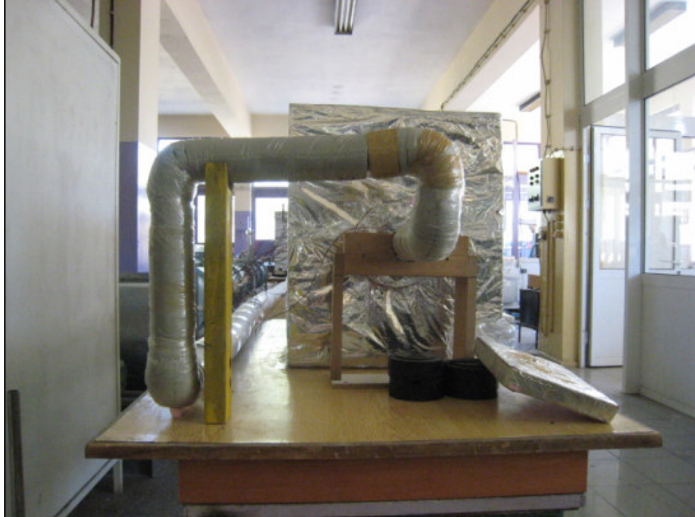
Figure 2.8 Pipe rise at the exit of the energy storage unit
