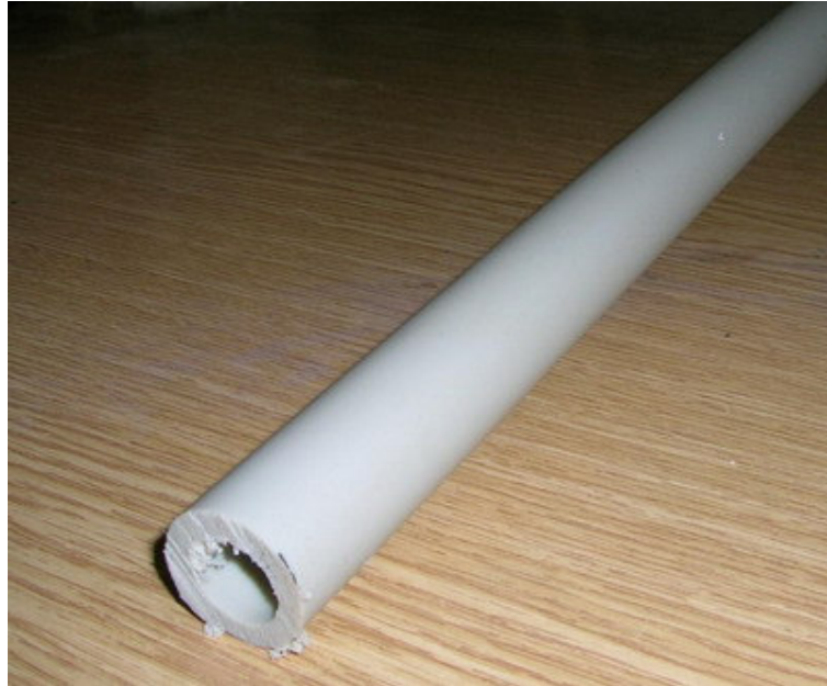
Figure 2.9 The pipe used for the flow of the HTF
