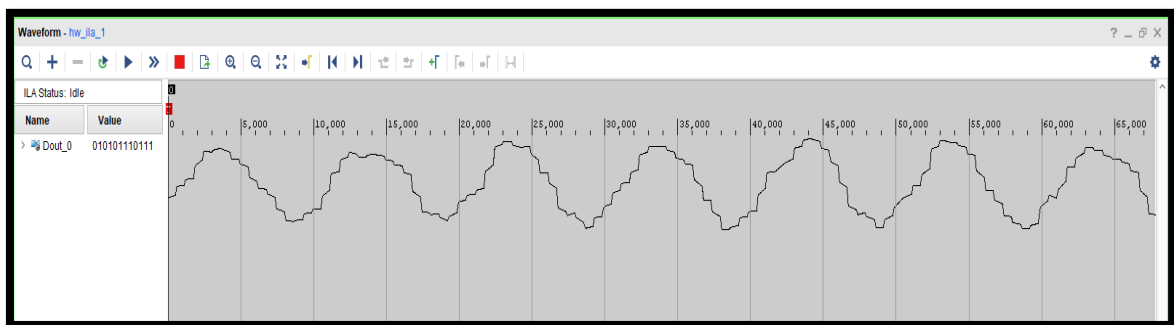
Figure 6.1. 3-taps filtered signal displayed in ILA
