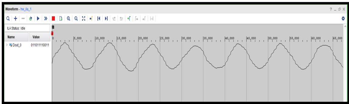
Figure 6.4. 8-taps filtered signal displayed in ILA
