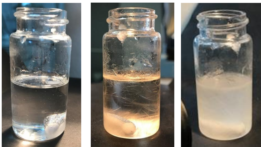
Figure 3.8. Changes of the mixture of \text{ZnCl}_2 -Urea and reline mixture in 1:1 molar ratio.
