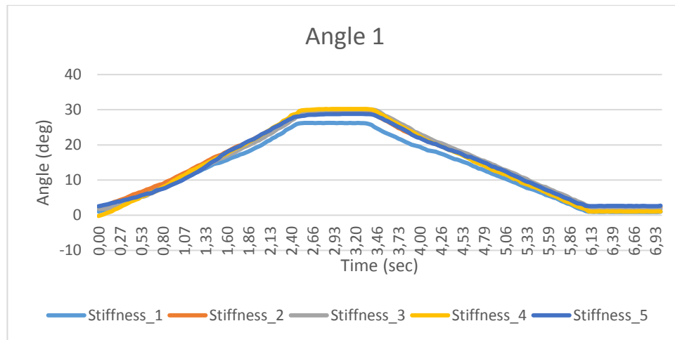
Figure 30: Joint MP angles for 5 different silicon fingers (experimental results)
