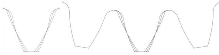
Figure 4.43 Root fillets and root regions for cases of ST-SR2, ST-SR3 and ST-SR4 (Having different symmetric pressure angles with limiting symmetric cutter tip radii coefficients)
