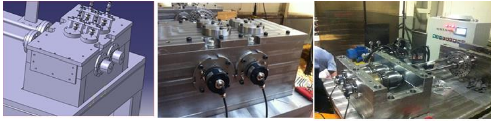
Figure 7.19 Encoder mounted on test rig shafts
