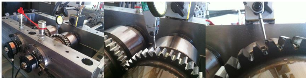
Figure 7.20 Calibrations of encoders by using dial indicator
