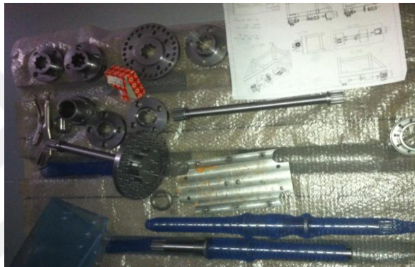
Figure 7.5 Torsional rods and multi-hole couplings
