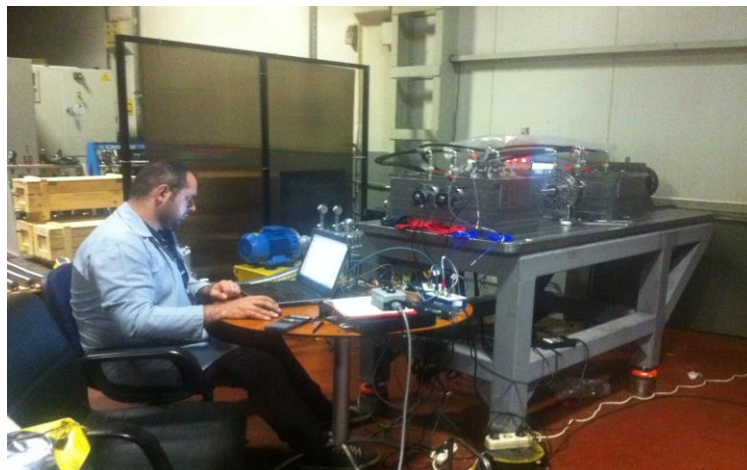
Figure 7.35 Conducting pretests of static transmission error measurements
