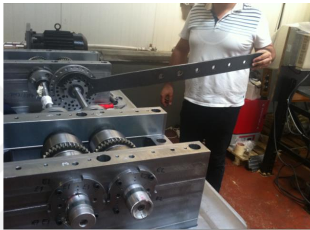
Figure 7.12 Designed and manufactured torque wrench for test rig
