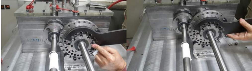
Figure 7.14 Loading by torque wrench on couplings and inserting pins-2
