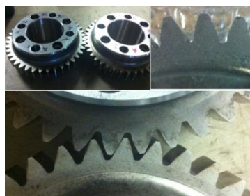
Figure 7.56 Asymmetric tooth profile spur gear pair of Case A22 (D30C20)
