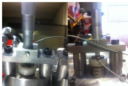
Figure 7.27 Positioning and calibration of Eddy current sensors by using micrometer
