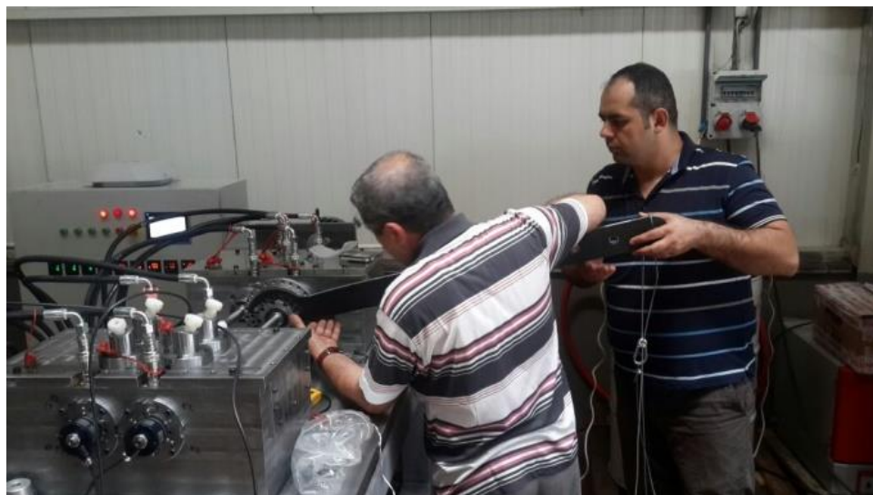
Figure 7.13 Loading by torque wrench on couplings and inserting pins-1
