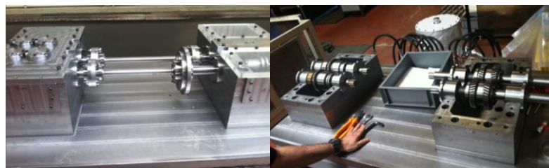
Figure 7.3 Test and slave gearboxes of test rig
