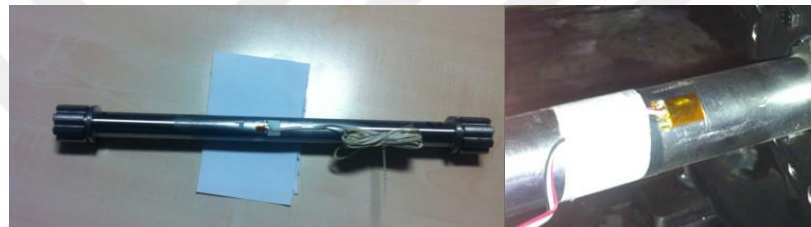
Figure 7.8 Strain gauges mounting on torsional rod
