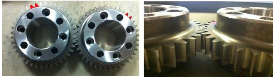
Figure 7.60 Asymmetric spur gear pair of Case A22
