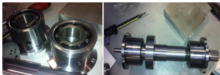
Figure 7.4 Bearing and housings of test and slave gearboxes
