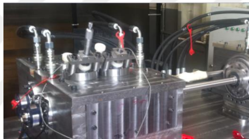
Figure 7.25 Positioning of Eddy current sensors on test rig
