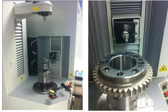
Figure 7.57 Measurement of tooth surface topology of gear pair (Case A22)
