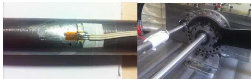
Figure 7.9 Strain gauges on torsional rod
