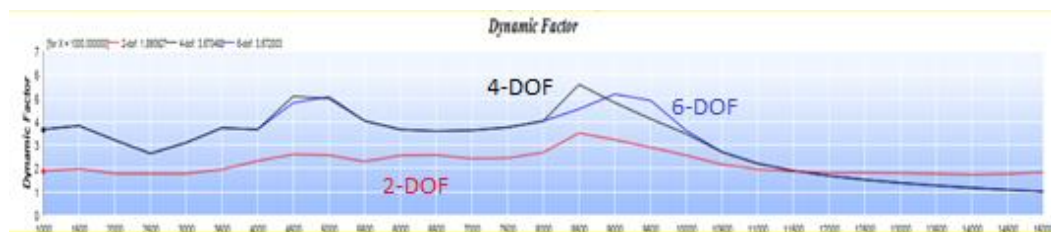
Figure 9.29 DF vs rpm for 2-DOF, 4-DOF and 6-DOF models
