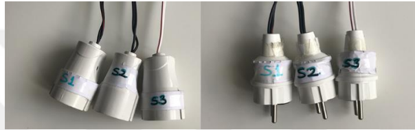
Figure 3.9. Plugs of the sensors (3 female plugs for connection to the line of luminaires, 3 male plugs for connection to the grid).
