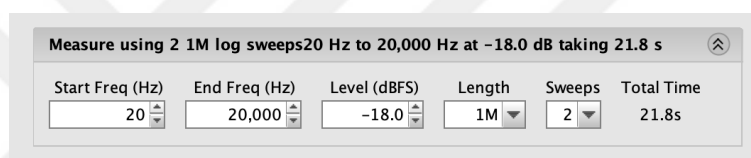
Figure 3.1 : Frequency sweep settings.
