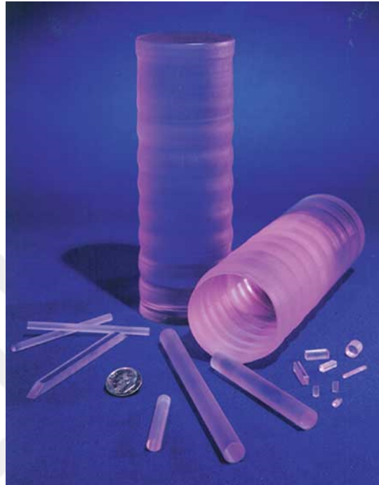
Figure 2.2: Different Nd:YAG Crystal Geometries [4]
