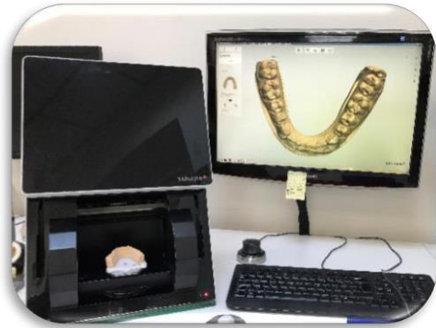
Figure 5.10. Digitizing the models and convert them to STL format
