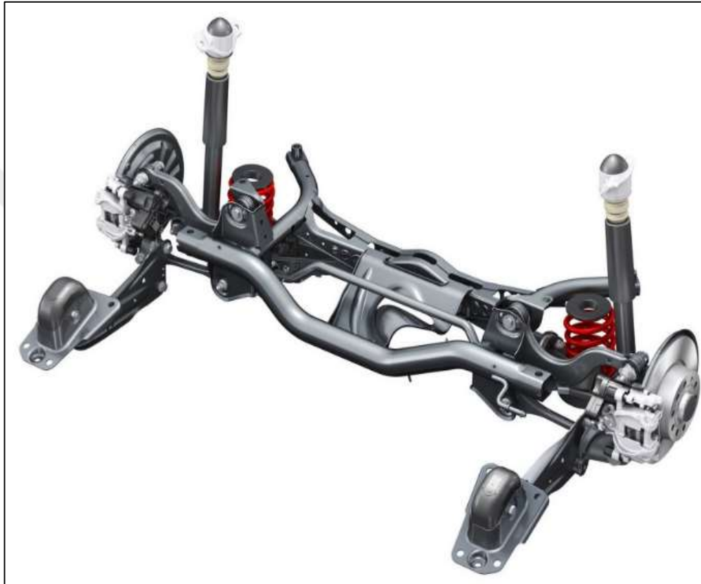
Figure 2.6: Multi-Link suspension system.
