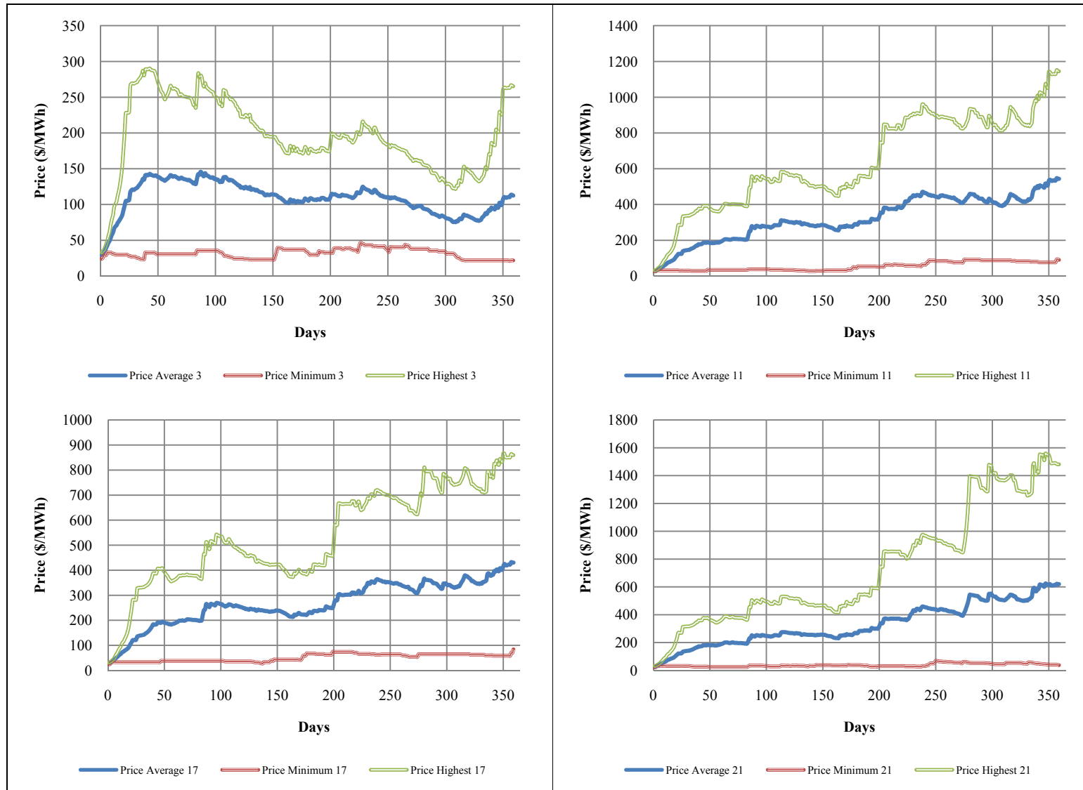
Figure 4.37. Impacts of transmission line capacities on electricity sales prices at the selected time intervals (AC OPF case).
