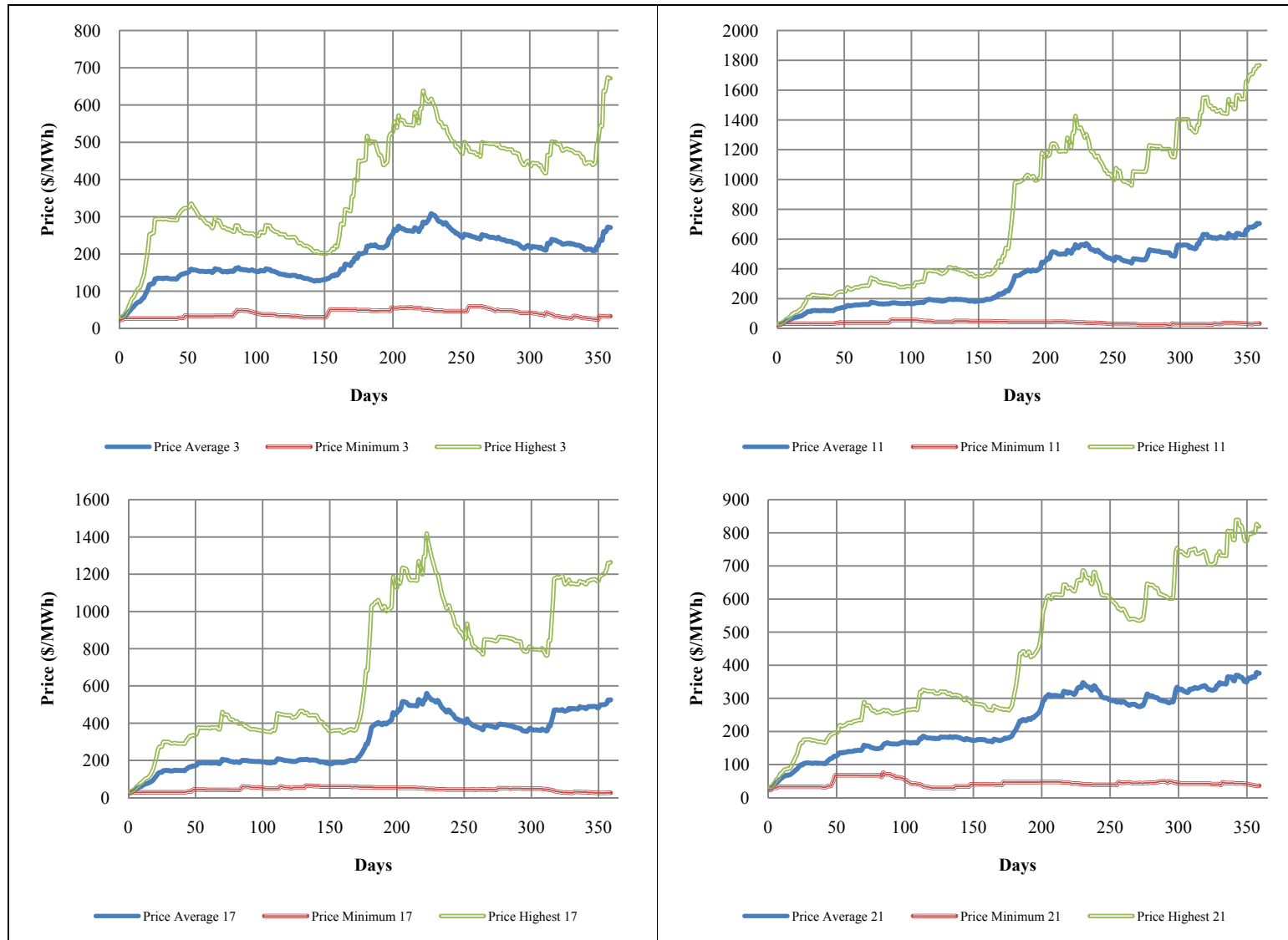
Figure 4.44. Impact of the combined bidding strategies on electricity prices at the selected time intervals (AC OPF case).
