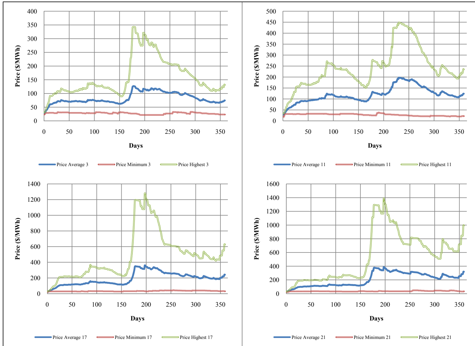
Figure 4.45. Impact of the demand shift on electricity prices at selected time intervals (AC OPF case).
