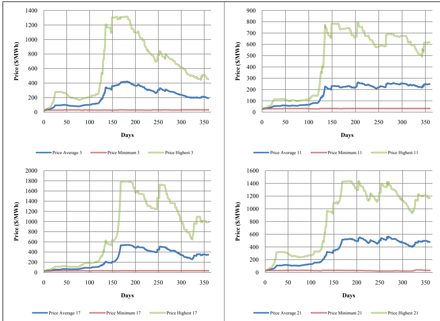
Figure 4.58. Impact of the NSGB5 scenario on electricity prices at the selected time intervals (AC OPF case).
