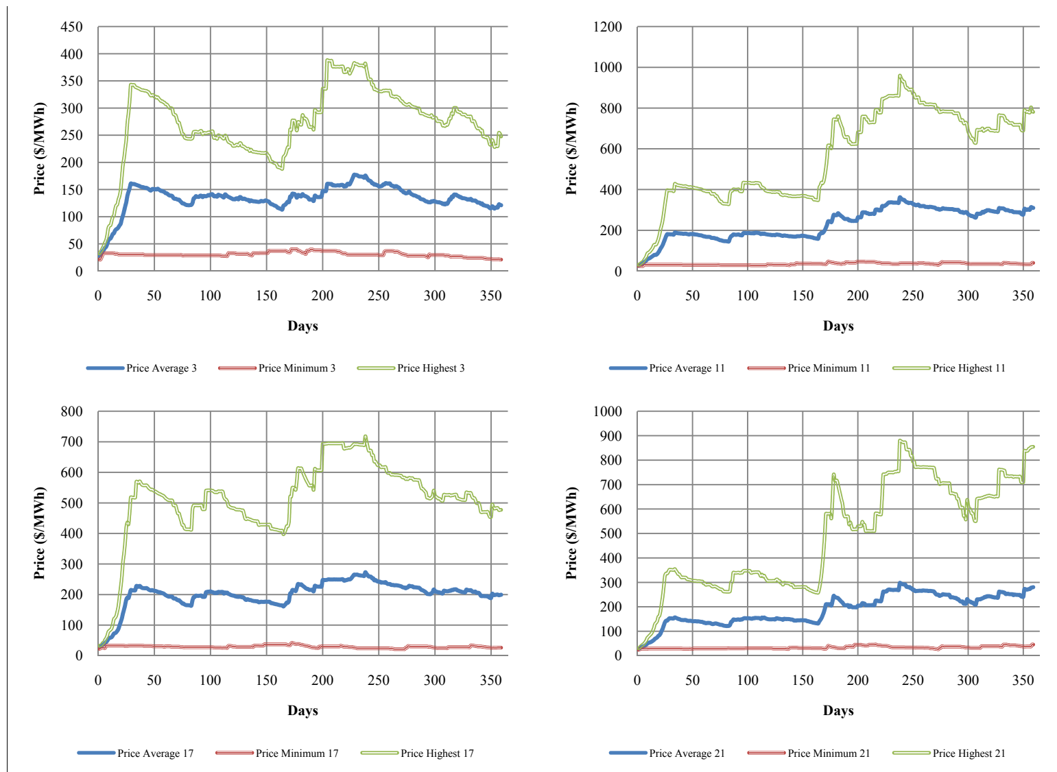
Figure 4.42. Impact of the Market Power based bidding strategy on electricity prices at the selected time intervals (AC OPF case).
