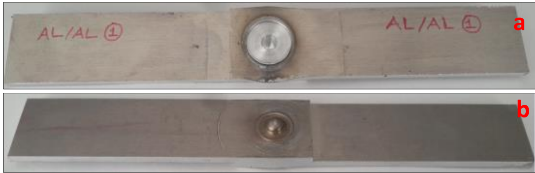
Figure 4.3 Welded aluminum sheets (a) top view (b) bottom view (Personal archive, 2017)
