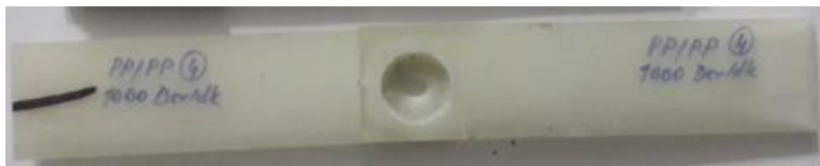
Figure 4.23 Welded PP GF%30 sheets (Personal archive, 2017)
