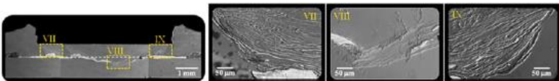
Figure 2.36 Cross-sectional views of weld part with tracer material using tool C, (a) similar Al welds; (b) Mg welds (Leon et al, 2016)
