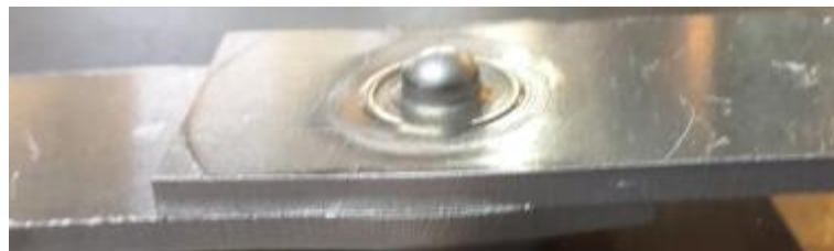
Figure 3.10 Illustration of dome protrusion shape on the welded sheets (bottom view) (Personal archive, 2017)
