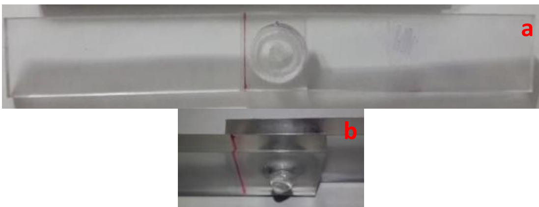
Figure.4.18 Welded PC sheets (a) top view (b) bottom view (Personal archive, 2017)
