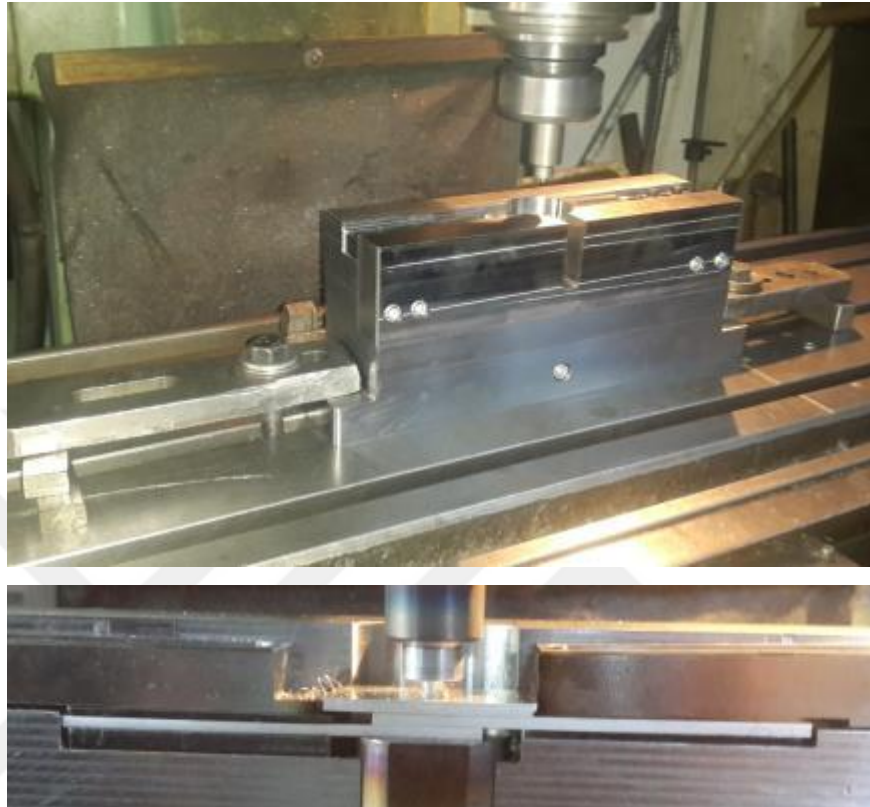
Figure 3.9 Illustration of the first step of the welding apparatus (Personal archive, 2017)
