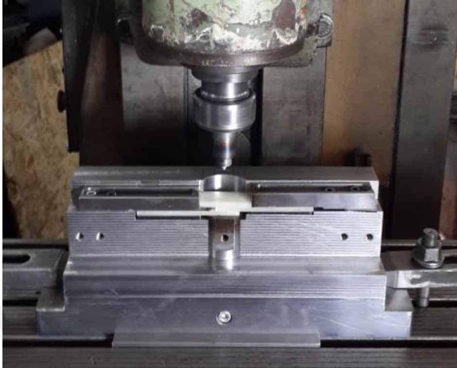
Figure 4.22 The position of PP 30% GF sheets in the welding apparatus (Personal archive, 2017)
