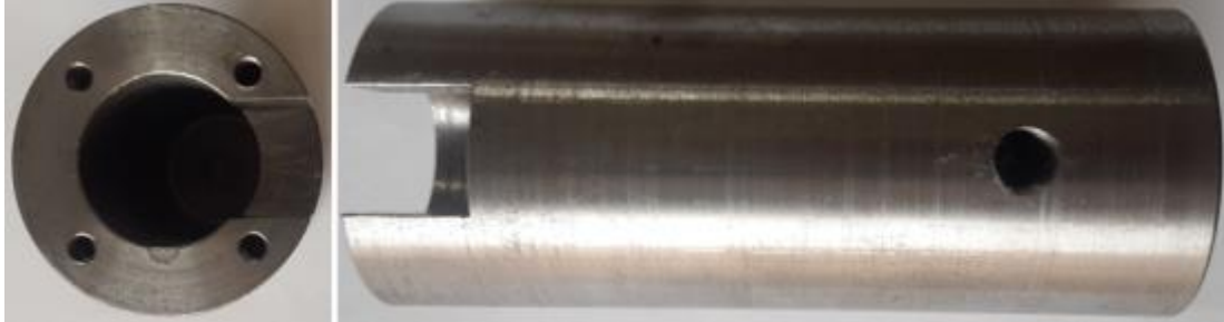
Figure 3.28 Manufactured mounting part for pre-heat kit (Personal archive, 2017)
