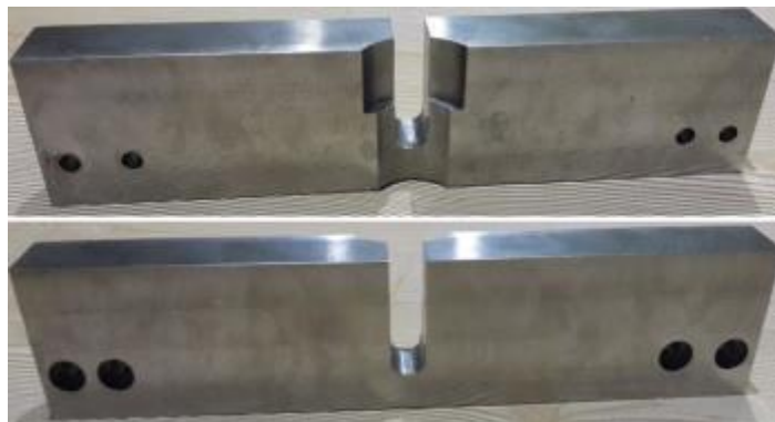
Figure 3.15 Manufactured main block additional part (Personal archive, 2017)
