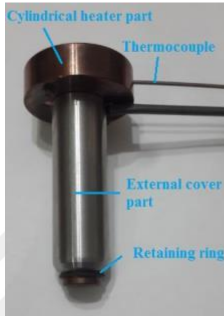
Figure 3.25 Manufactured pre-heat process kit (Personal archive, 2017)
