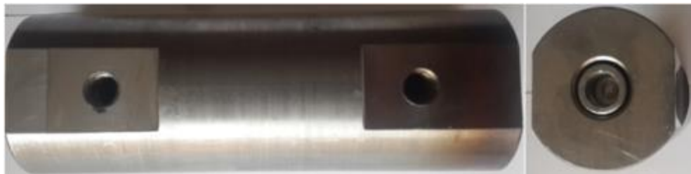
Figure 3.17 Manufactured cylindrical weld extrusion block (Personal archive, 2017)
