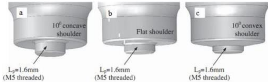
Figure 2.30 Schematic of FSSW tool shoulder geometries a) concave, (b) flat, (c) convex (Badarinarayan et al., 2009)
