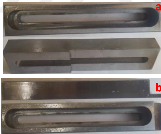
Figure 3.24 Produced right (a) and left (b) fixing parts (Personal archive, 2017)
