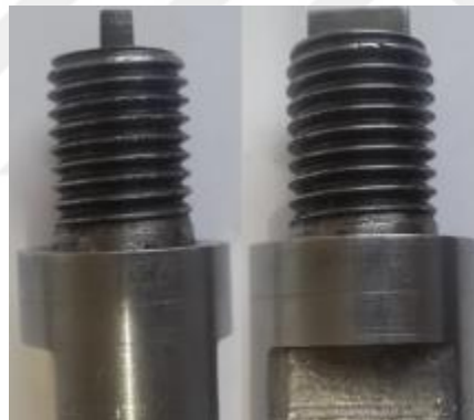
Figure 3.19 Produced shoulder-milling machine interconnection part (Personal archive, 2017)
