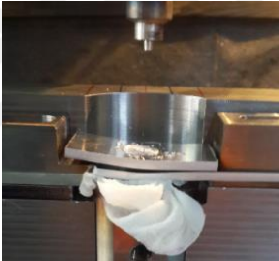
Figure 4.30 The welded sample of PP 30% GF - aluminum sheet (Personal archive, 2017)
