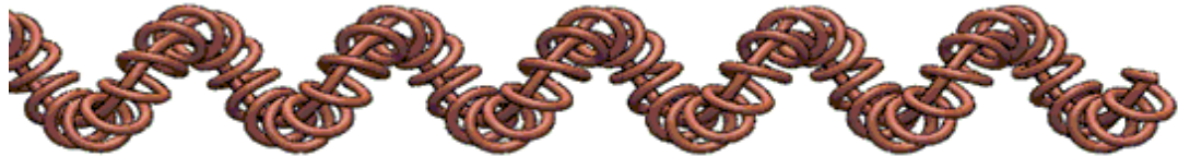
Figure 4.1 Circular wire coil insert around circular wire coil type one
