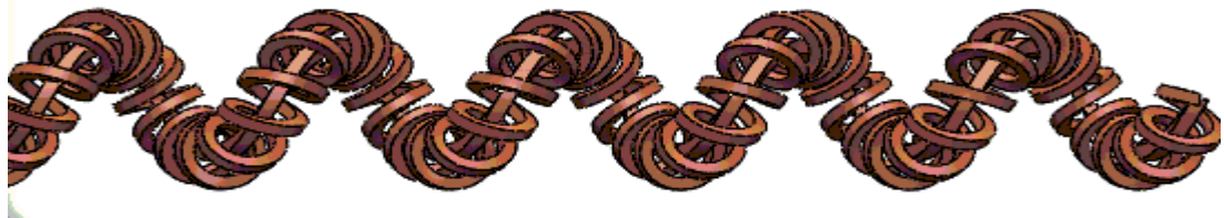
Figure 4.19 Square wire coil insert around Square wire coil type one
