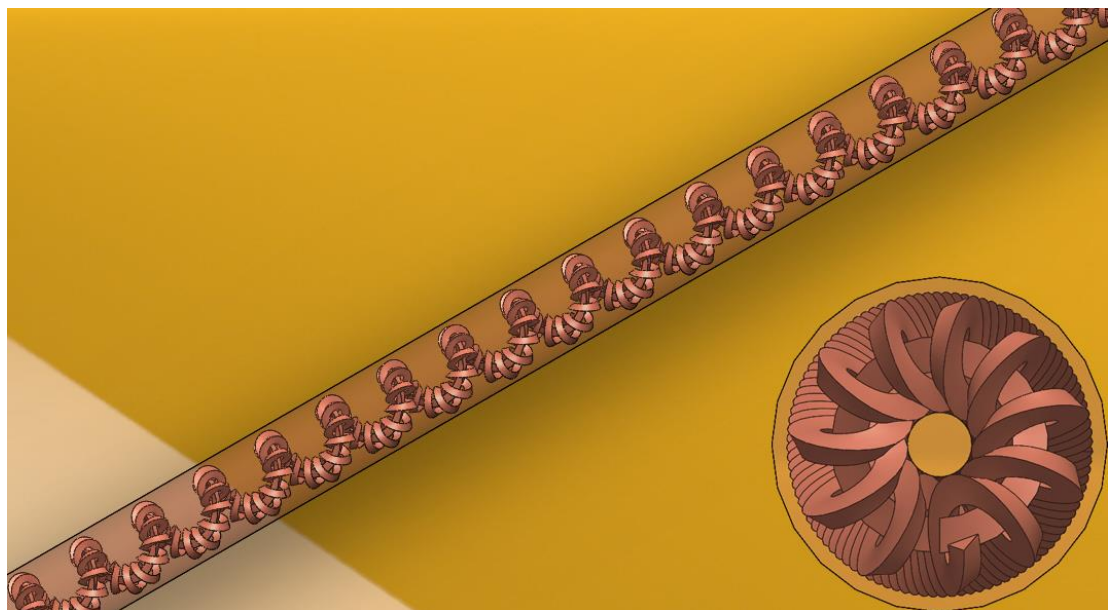
Figure 4.36 Geometry of the triangular wire coil insert around triangular wire coil in tube fitted type one
