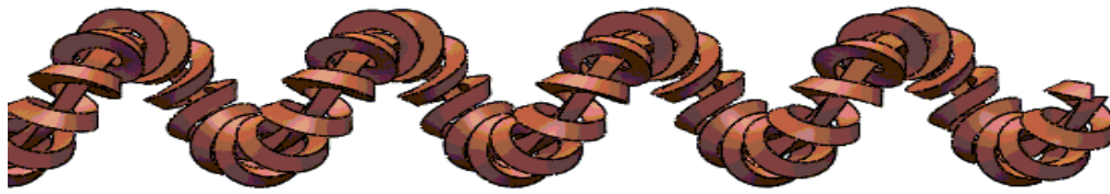
Figure 4.35 Triangular wire coil insert around triangular wire coil type one
