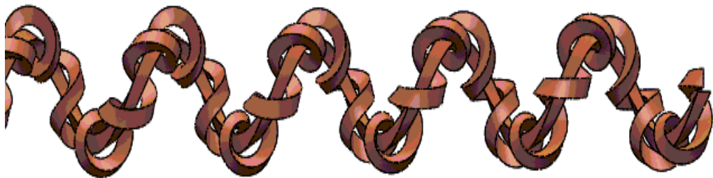
Figure 4.44 Triangular wire coil insert around triangular wire coil type two
