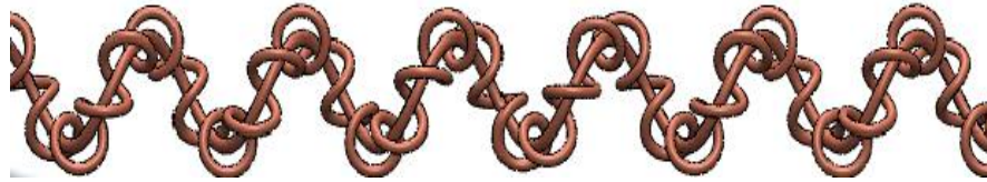
Figure 4.10 Circular wire coil insert around circular wire coil type two
