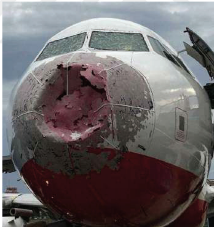
Figure 1.10. Airplane damaged by nose and windshield during hailstorm (Source: QHA, 2017)
