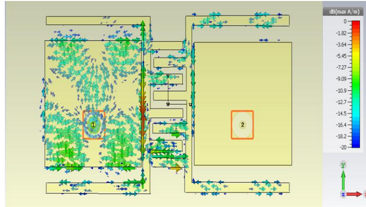
Figure 4.41 Surface current distributions at 10.3 GHz with LSCW structure
