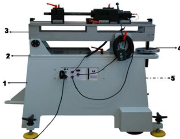
Figure 5.11 : Schematic view of shooting weapon (1) main body and subframe compartment; (2) upper carrier section; (3) crib; (4) incremental adjustment; (5) side adjustment wheel.
