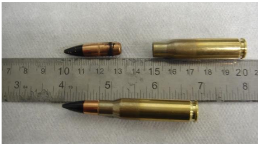
Figure 5.8 : The photo of the 7.62 × 51-mm NATO bullet with and without full metal jacket.
