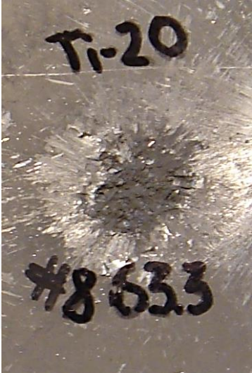
Figure 6.68 : The damage occurred on the Al backing alloy surface after the hit with the protection of 20 vol. Ti-LP added boron carbide composite tile which was spark plasma sintered at 1550 °C for 4 min under a pressure of 40 MPa in vacuum.
