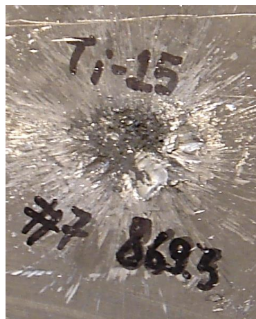
Figure 6.67 : The damage occurred on the Al backing alloy surface after the hit with the protection of 15 vol. Ti-LP added boron carbide composite tile which was spark plasma sintered at 1550 °C for 4 min under a pressure of 40 MPa in vacuum.
