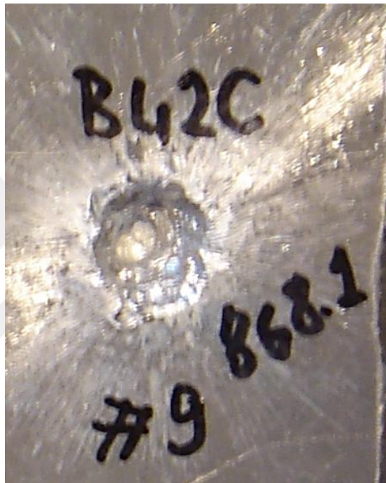
Figure 6.61 : The damage occurred on the Al backing alloy surface after the hit with the protection of 2 vol. % C-black added boron carbide tile which was spark plasma sintered at 1550 °C for 4 min under a pressure of 40 MPa in vacuum atmosphere.
