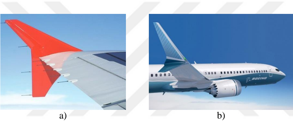
Figure 2.7: a) Fence winglet on Airbus A319, b) Combined winglet (blended&fence) on Boeing 737 MAX.
