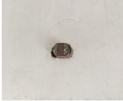
Figure 4.4 Photocell sensor connected to the smart home system.
