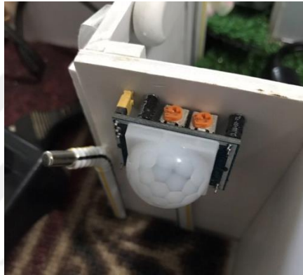
Figure 4.5 PIR sensor connected to the smart home system.
