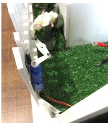
Figure 4.1 Servo motor connected to the smart home system.
