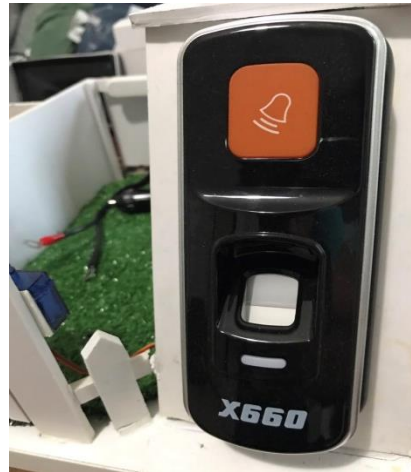
Figure 4.2 Biometric fingerprint / RFID card reader connected to smart home system.
