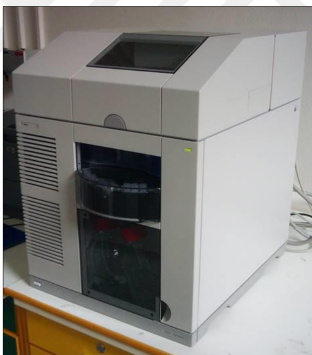
Figure 3.1. Agilent G1600AX 3D Capillary Electrophoresis instrument
