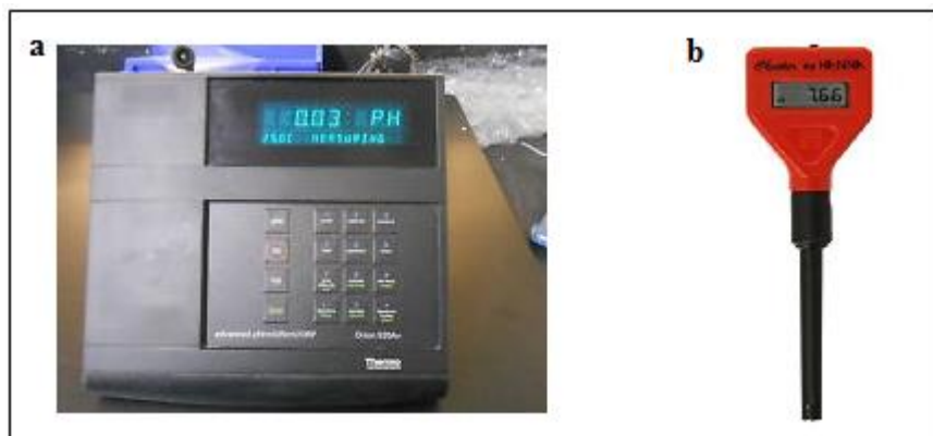
Figure 3.2. a) Thermo Electron Orion 720A pH meter and b) Hanna HI98103 Checker pH tester.
