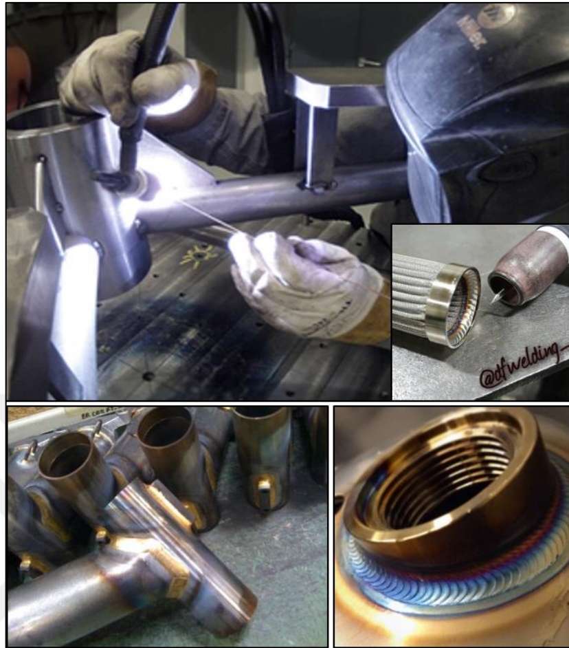
Figure 4.4. Some applications on TIG welding.
