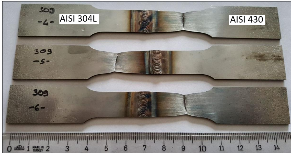
Figure 6.17. Macro photographs of the refraction areas of the Standard A welded tensile specimens combined with ER309 additional wire.
