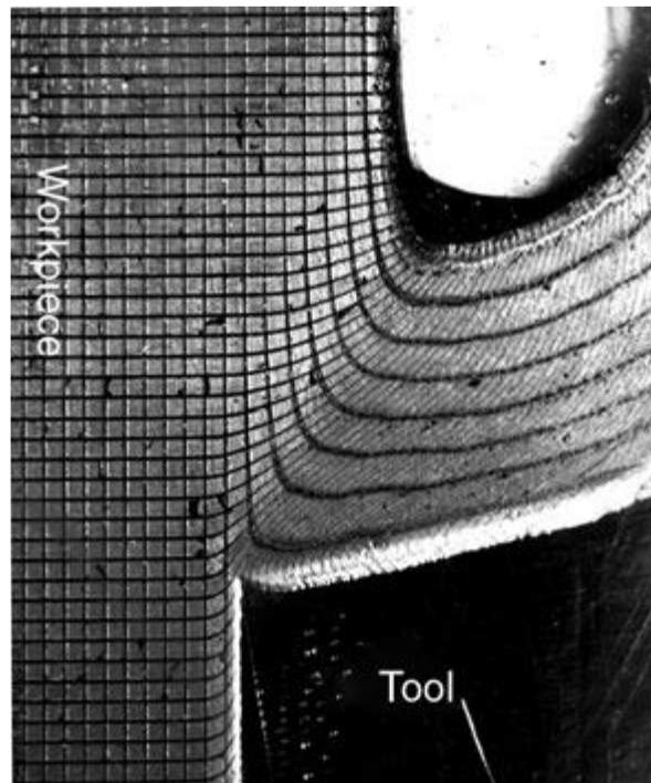
Figure 2.10 : Deformation representation of workpiece.
