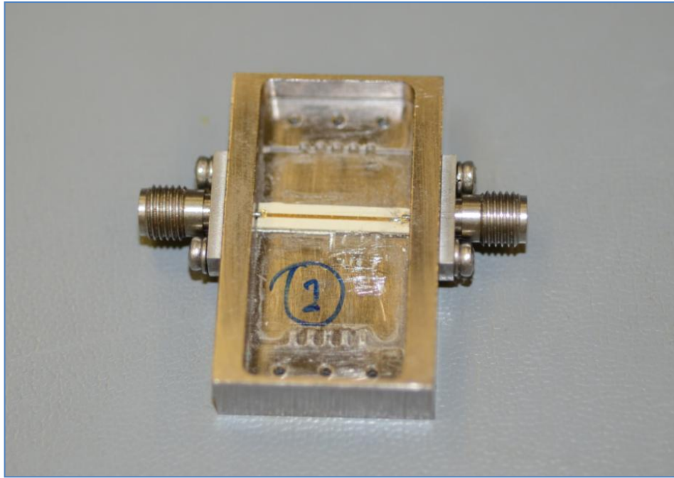
Figure 3.22 Photograph of measured transmission lines and connectors
