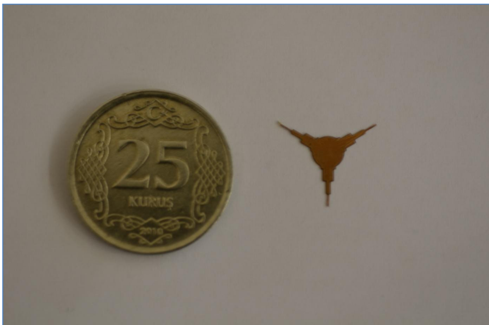
Figure 3.17 Berilium Copper (CuBe 2 ) Y-junction
