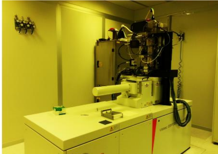
Figure 3.3 Vistec EBPG5000+ES 100 kV electron beam lithography system at SUNUM.
