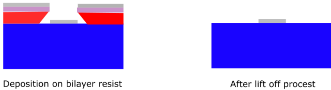
Figure 3.7 Schematic of lift off process
