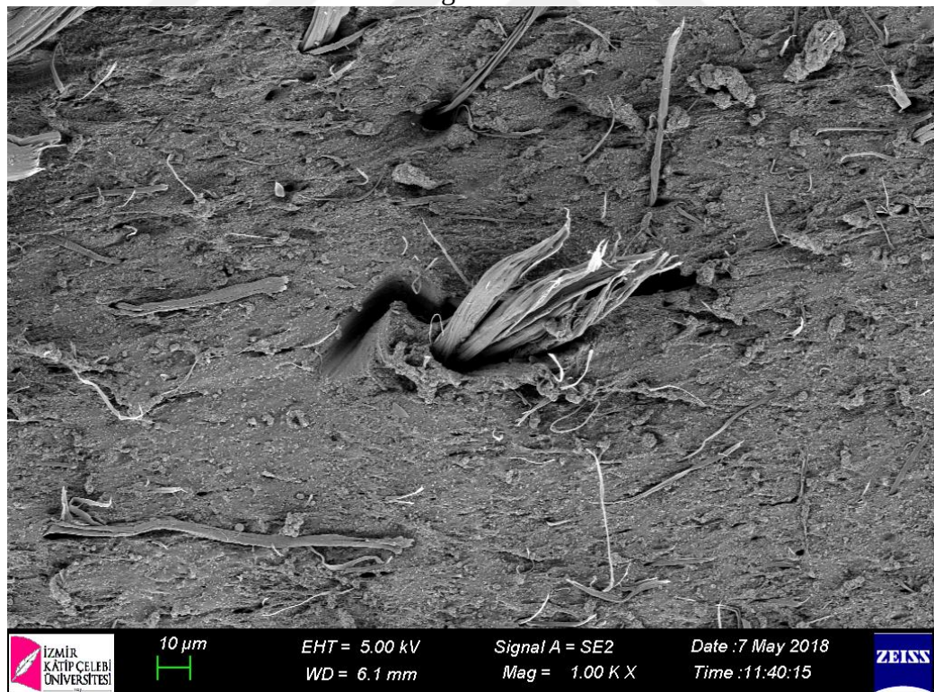
Figure 3.30: SEM analysis of EPDM rubber mixture with non-treated aramid fiber
