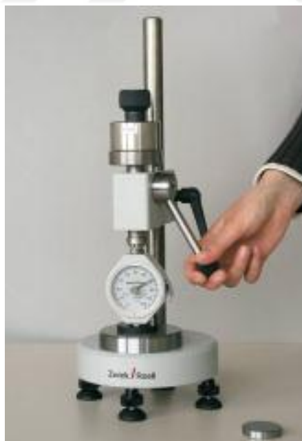
Figure 2.4: Zwick hardness test instrument [40]
