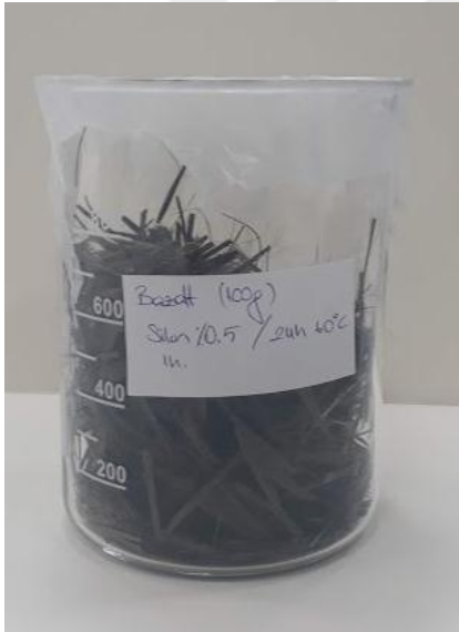
Figure 2. 26: Silane bonding agent solution with a Ph value of 4,5
