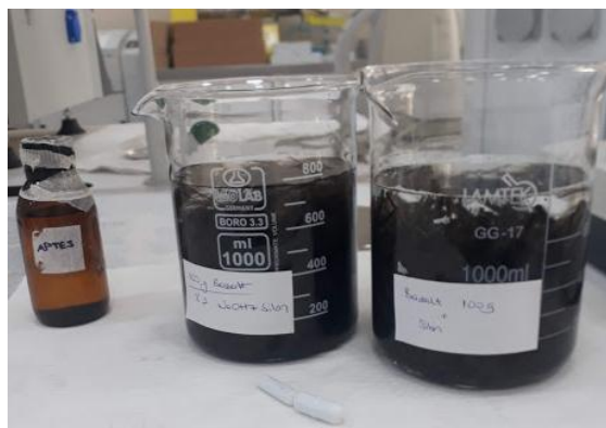
Figure 2.29: Silane and NaOH treated basalt fiber.
