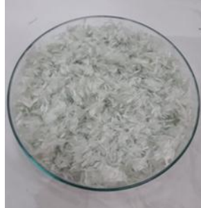
Figure 2.24: Glass fiber after alkali solution treatment
