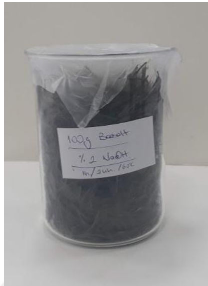
Figure 2.28: NaOH applied, dried basalt fiber
