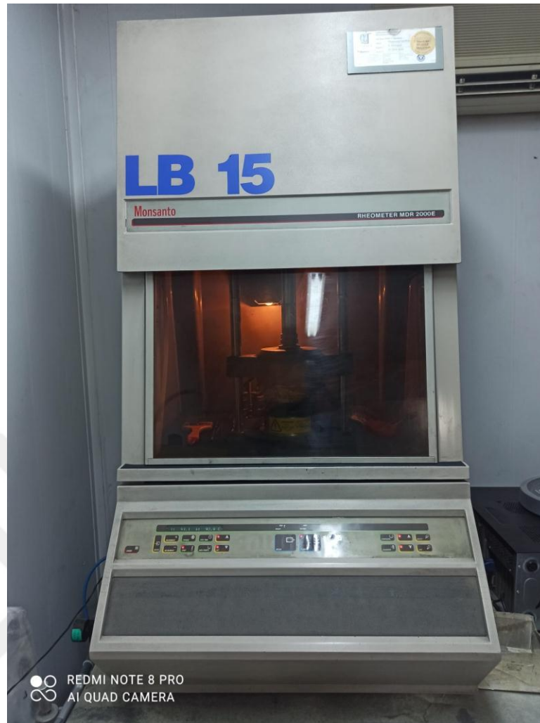
Figure 2.1: Alpha MDR 2000 Moving die Rheometer with computer
