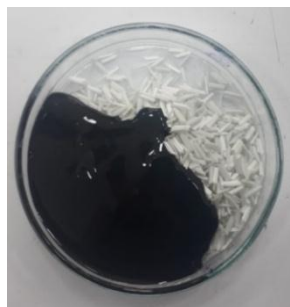
Figure 2.23: EPDM solution and Glass Fiber
