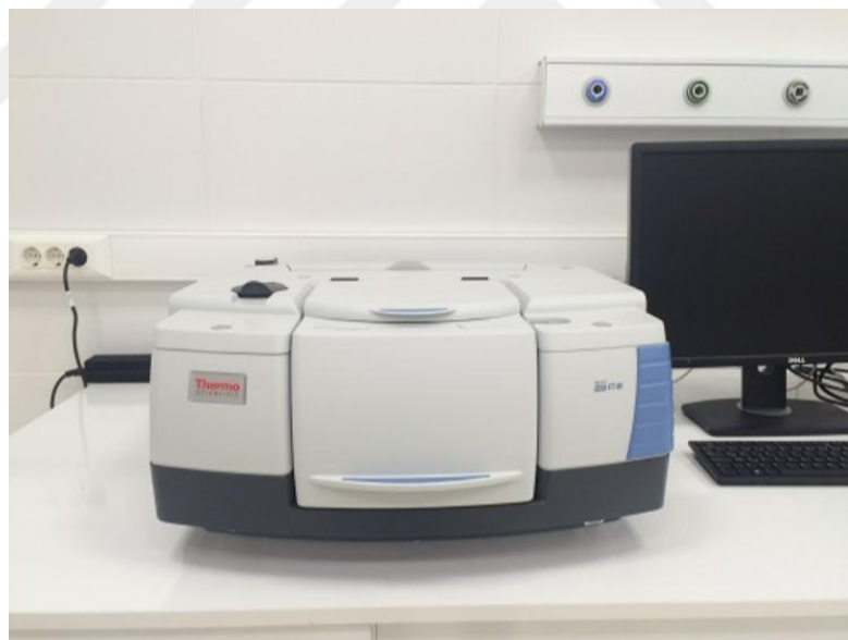
Figure 2.10: FTIR test machine
