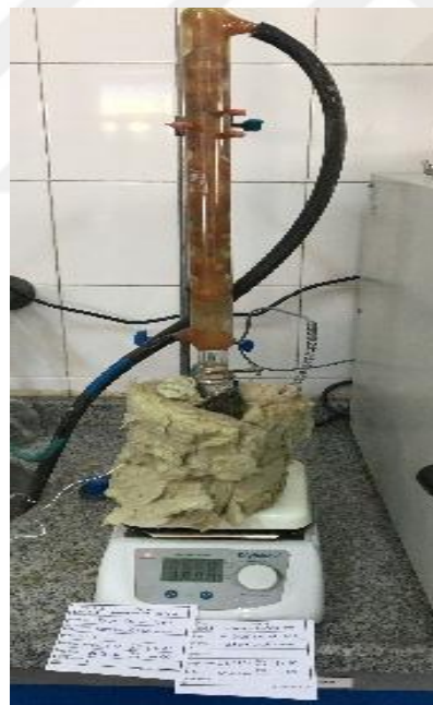
Figure 2.6: Reflux condenser for coolant ageing
