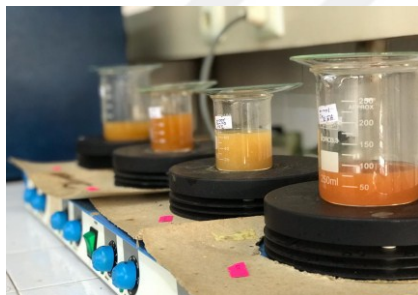
Figure 4.10: (a) \text{AgNO}_3 solution, water extract of plant before reduction and silver dispersion formed after reduction, (b) Ag-CoNPs with CoNPs (WE), (c) Ag-CoNPs formed in different concentration (WE), (d) \text{AgNO}_3 with methanol extract (ME), (e) \text{AgNO}_3 with ethanol extract (EE), (f) AgNPs formed after reduction (ME), (g) \text{Co}(\text{NO}_3)_2 \cdot 6\text{H}_2\text{O} with extract (EE), (h) Ag-CoNPs formed after reduction of both (ME), (EE), (i) AgNPs formed after reduction of (EE).
