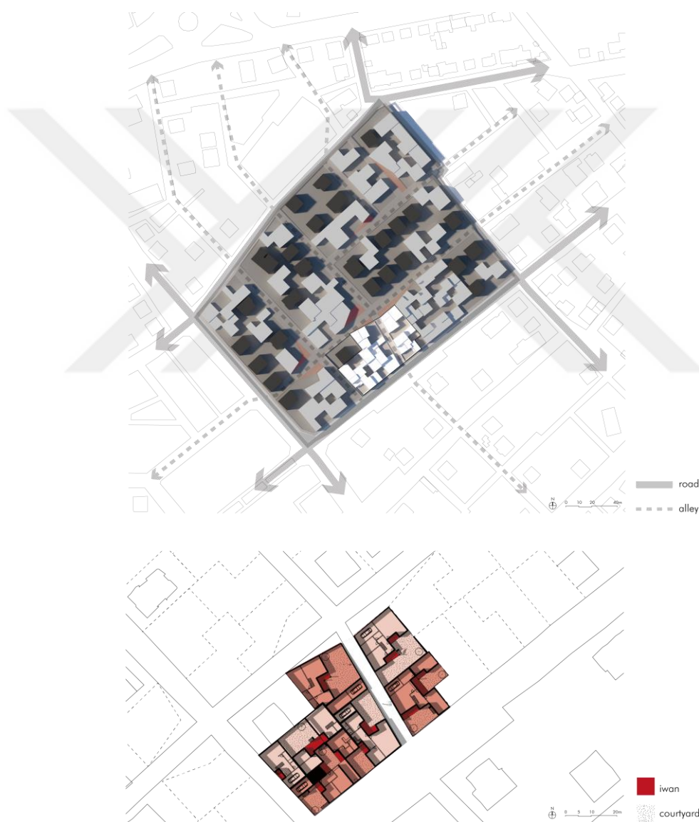
Figure 4.93. A possible urban composition based on generative typomorphological urban design code: the plan of the ensemble within the proposed street layout (above) and a close-up plan within the ensemble (below). Note that different shades of color indicate different plots.
