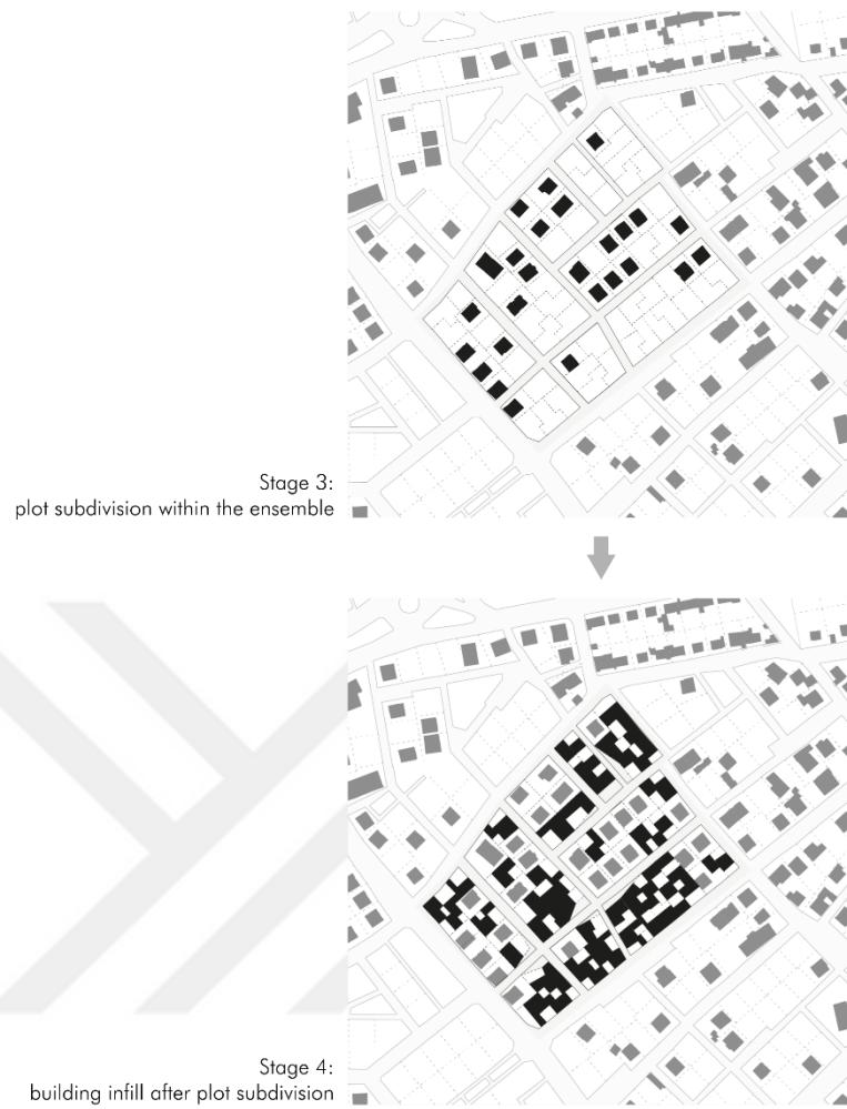
Figure 4.92. Stages 3 & 4: plot subdivision and building infill.
