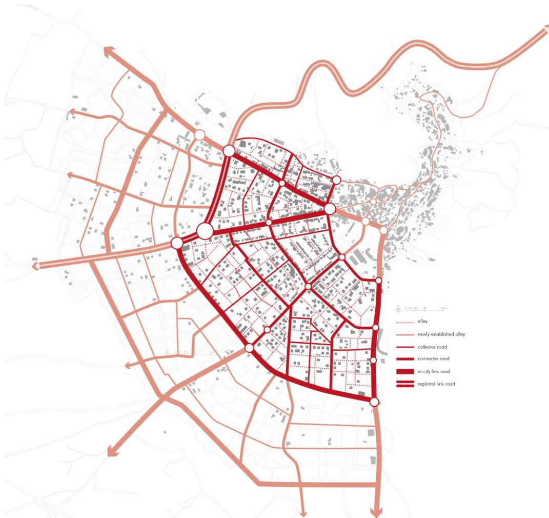
Figure 4.88. The proposed street network in the new settlement area. The existing street layout is not changed except several alleys passing through existing building-blocks. Note that in the scope of this study, only the area reaching up to the in-city and regional link road (the bright colored area) is studied in terms of alleys.
