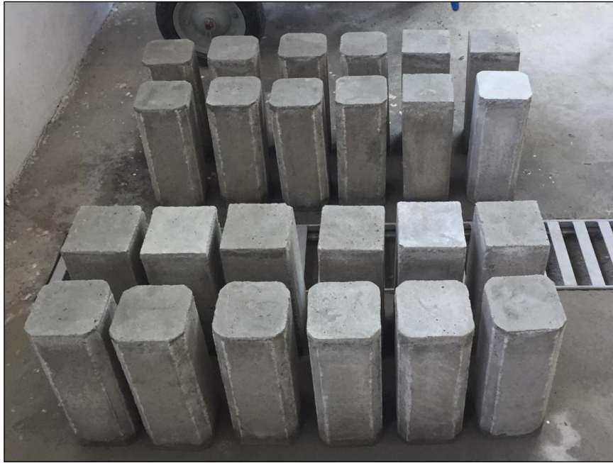
Picture 3.7. Concrete specimens after capping the ends
