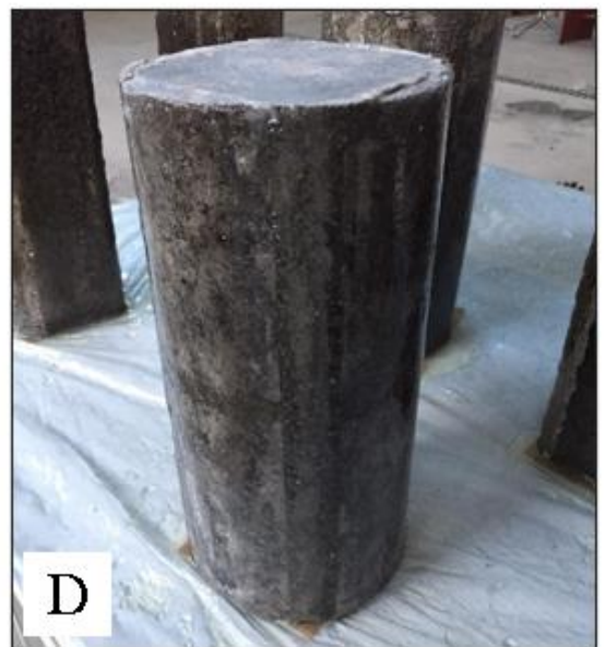
Picture 3.10. Steps of implementing the shape modification technique for the rounded-corners of the core, a) top view for the core and the concrete segments, b) applying the epoxy on the surface of the specimen and the concrete segment, c) attaching the specimens on the surface of the core, and d) the final shape of the specimen.
