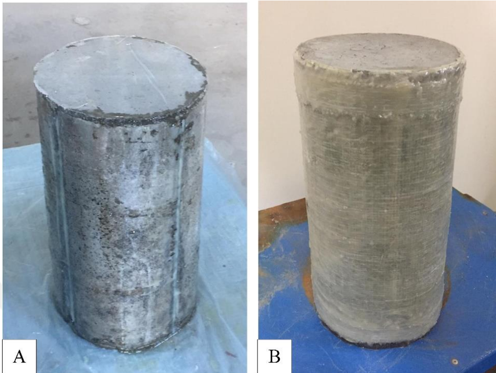
Picture 3.15. CCF group, a) applying the epoxy primer, and b) wrapping the GFRP sheet.
