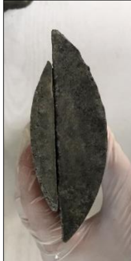
Picture 3.6. Size difference between the concrete segment of the proposed shape modification method and the previous shape modification method
