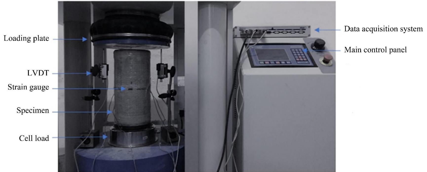
Picture 3.20. Test set-up
