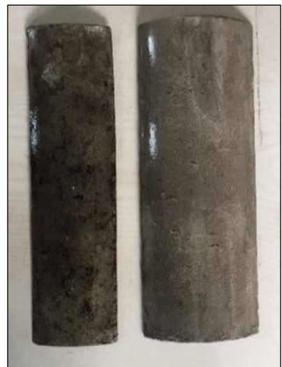
Picture 3.6. Size difference between the concrete segment of the proposed shape modification method and the previous shape modification method
