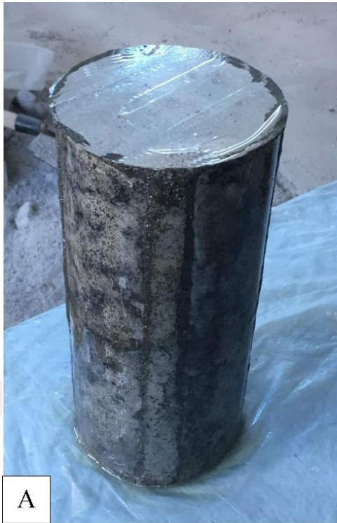
Picture 3.17. CRCP1 group, a) applying the epoxy primer, and b) wrapping the GFRP rings.
