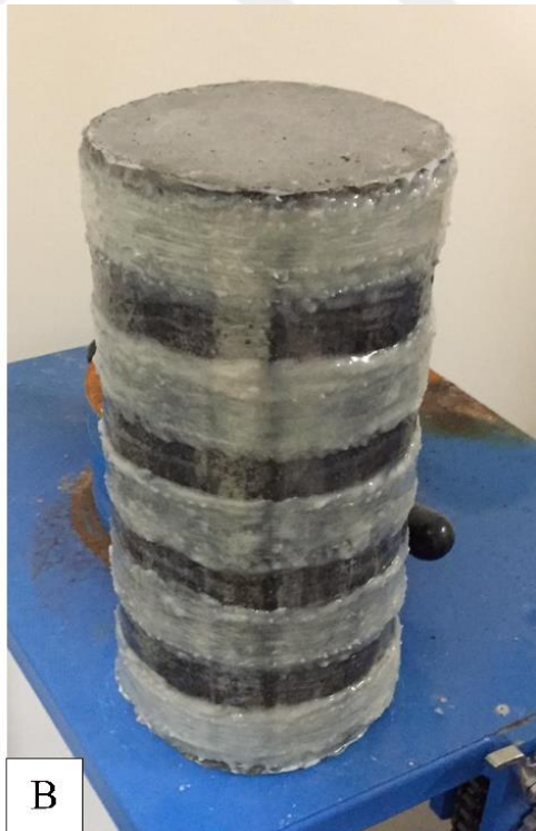
Picture 3.18. CRCP2 group, a) applying the epoxy primer, and b) wrapping the GFRP rings
