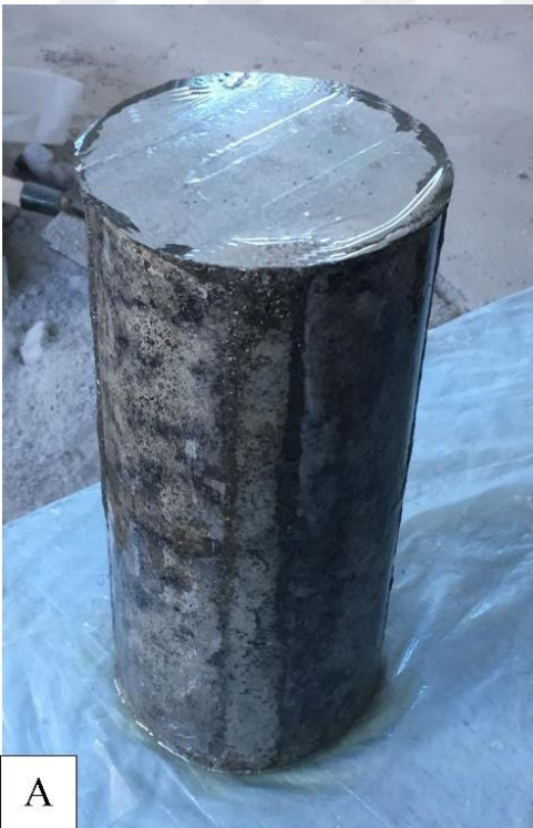
Picture 3.18. CRCP2 group, a) applying the epoxy primer, and b) wrapping the GFRP rings
