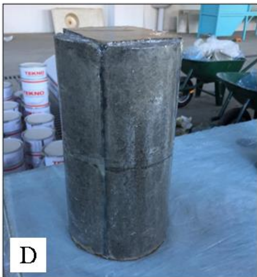
Picture 3.11. Steps of implementing the shape modification technique for the unrounded-corners of the core, a) top view for the core and the concrete segments, b) applying the epoxy on the surface of the specimen and the concrete segment, c) attaching the specimens on the surface of the core, and d) the final shape of the specimen.
