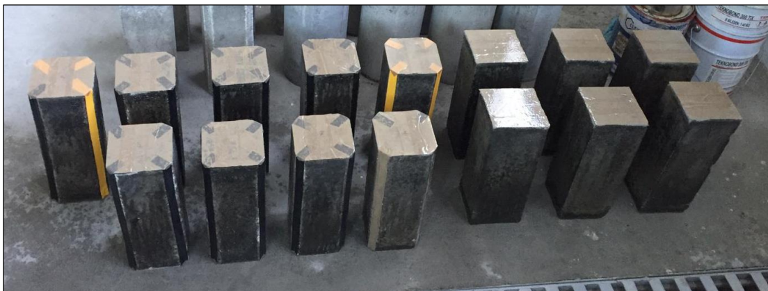
Picture 3.9. Concrete specimens after covering the ends and the corners
