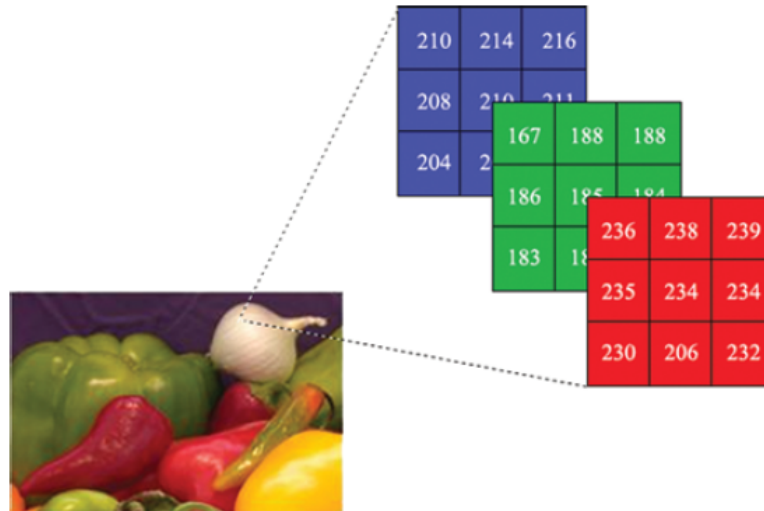
Figure 4.3 Pixels of a colour image (Sinecen, 2016)
