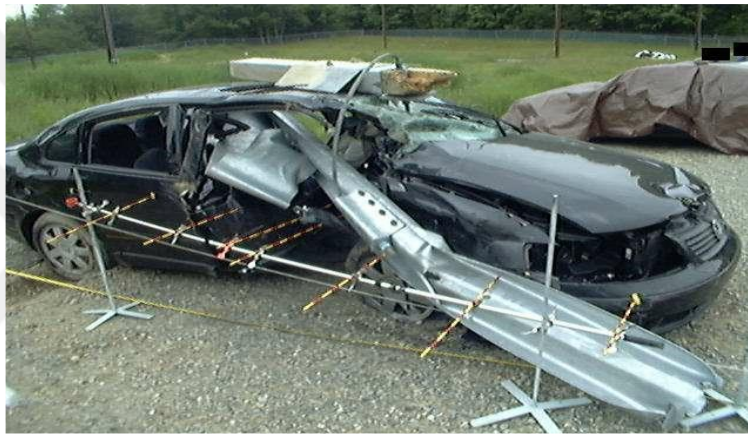
Figure 3.9. Steel guardrails terminal hazards [87].
