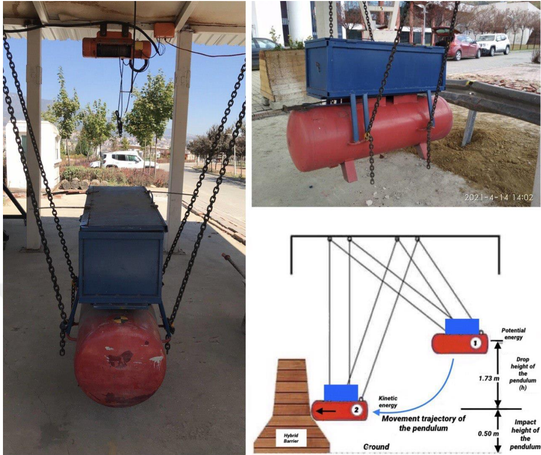
Figure 5.9. Experimental pendulum crash system.
