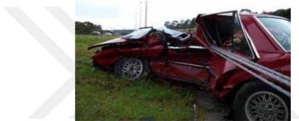
Figure 3.12. Under riding of vehicle due to wire rope [13].
