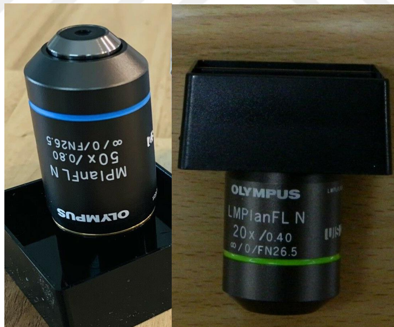
Figure 6-3- 50x and 20x Olympus lens to extract grit geometrical properties
