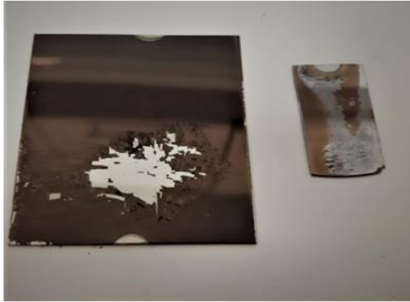
Figure 12. Samples for first magnetron sputtering trials. \text{Al}_{67}\text{Ti}_{33}\text{N} on SS substrate (left) and \text{Al}_{50}\text{Ti}_{50}\text{N} on Si(100) substrate (right).
