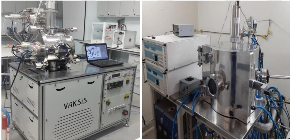
Figure 11. Vaksis Magnetron Sputterer in ODTÜ and in-house manufactured Magnetron Sputterer in İTU.
