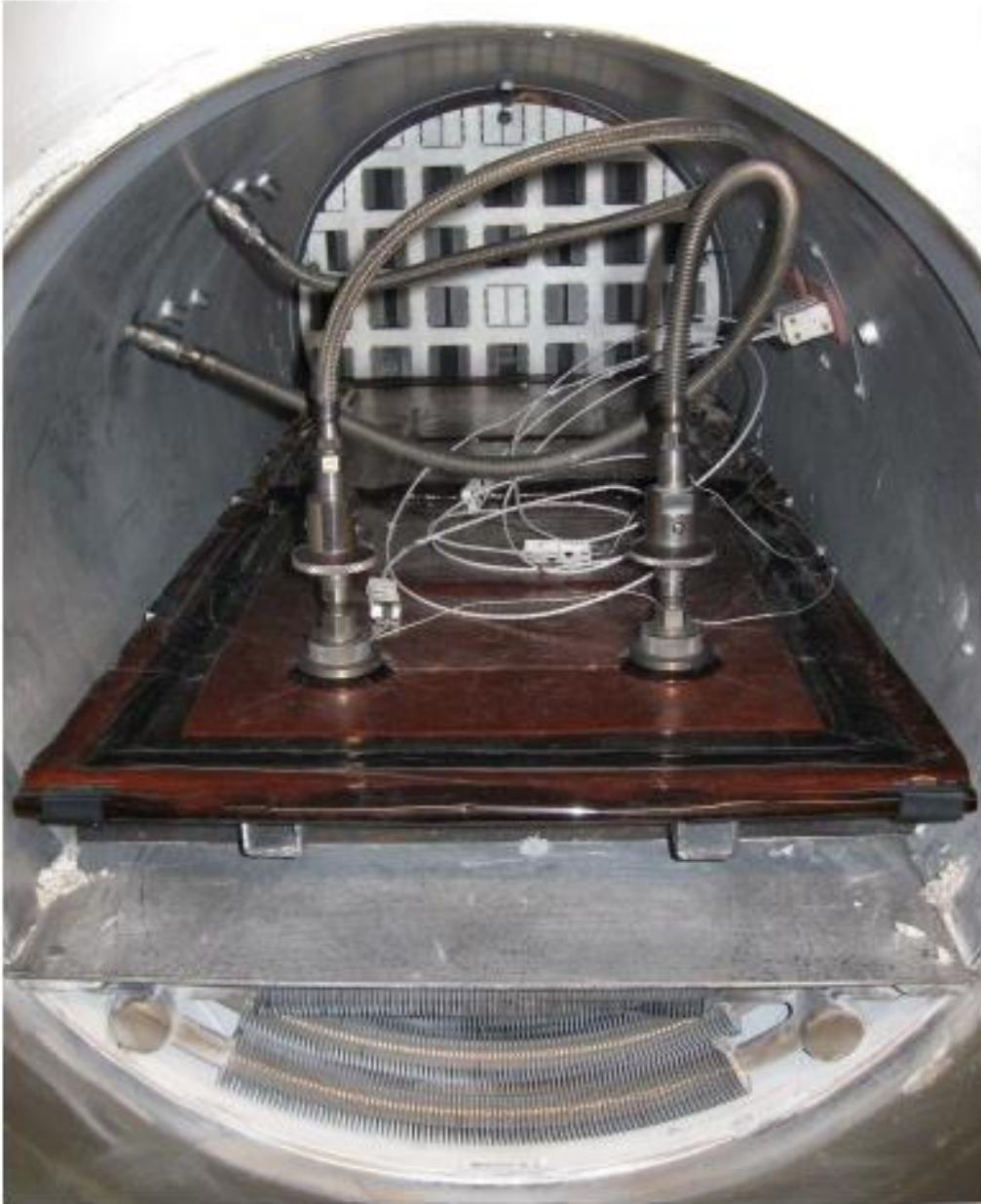
Figure 2.1 : An illustration for the vacuum bag in an autoclave.
