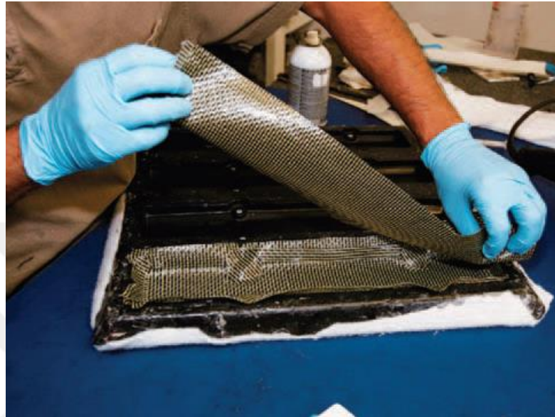
Figure 2.4 : Representation of prepreg hand lay-up.
