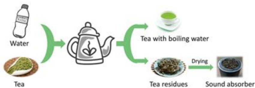
Figure 2.14 : Illustration of flow chart showing the steps to obtaining tea waste (Tang et al., 2020).
