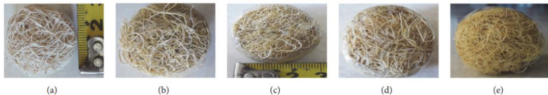
Figure 2.21 : Images of the sample: (a) raw CHF panel; and panels treated with addition of NaOH solutions at percentages of (b) 1%; (c) 2%; (d) 5%; (e) 8% (Sari et al., 2016).
