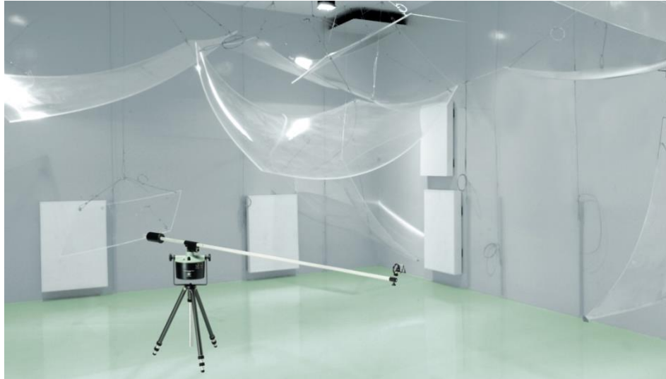
Figure 2.8 : The reverberation room used for measuring the sound absorption of a sample using sound source, the reflectors and microphones (Kuttruff, 2009).
