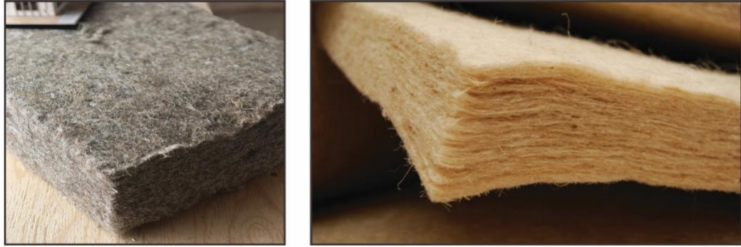
Figure 2.6 : Examples of porous absorbing materials made from natural fibers: hemp (left image) and kenaf (right image).
