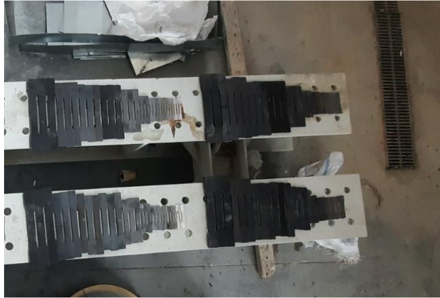
Figure 2.2. Test specimens with different thicknesses for S235JR.
