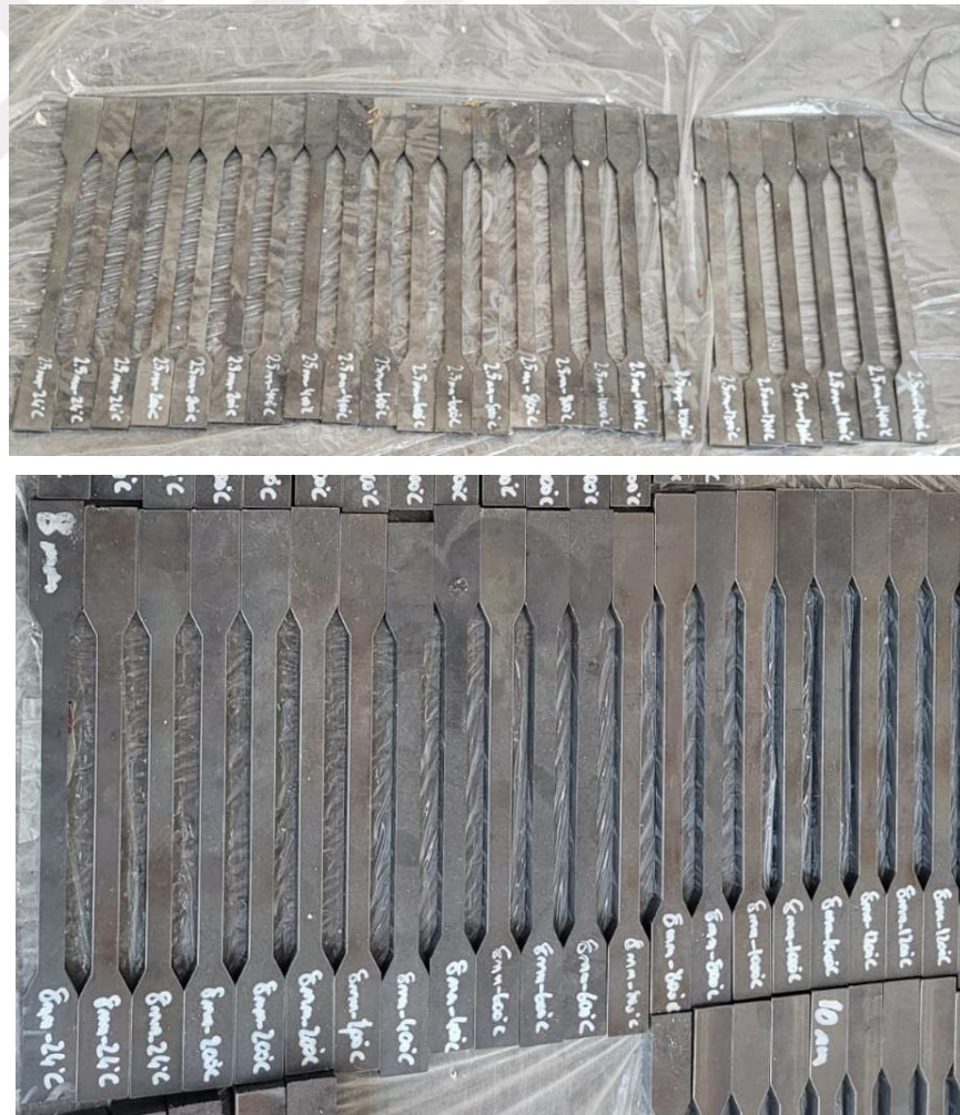
Figure 2.1. Test specimens with plate thicknesses of 2.5 mm and 8 mm for S700MC.
