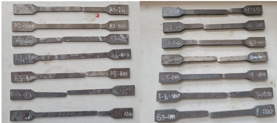
a) Failure modes of tension test specimens for S700MC steel grade
