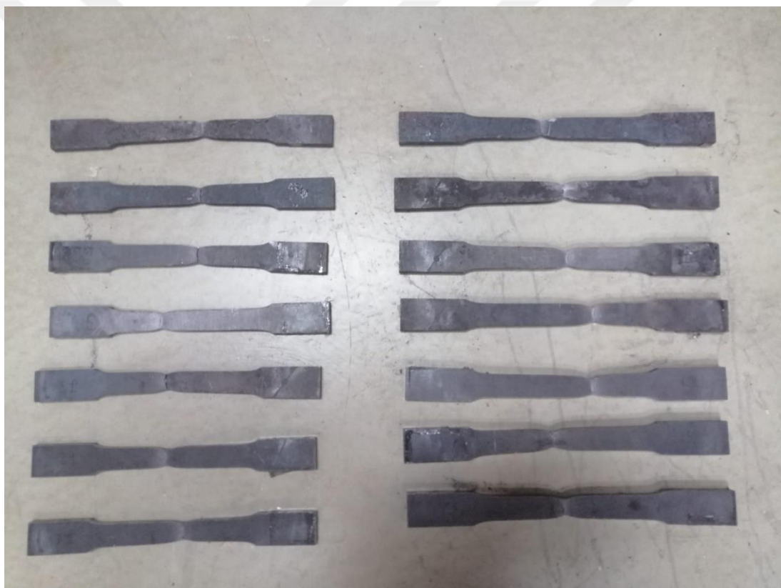
b) Failure modes of tension test specimens for S235JR steel grade
