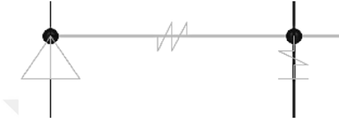
Figure 5.5. A link/support element in the FE model in SAP 2000.
