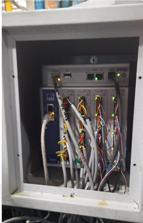
Figure 3.3 : Data acquisition device (HBM PMX).
