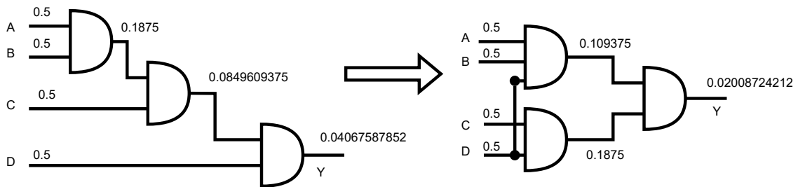
Figure 2.2. Logic restructuring of the Y=ABCD function.
