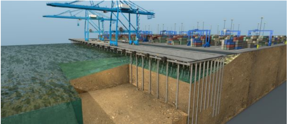
Figure 2.2. Typical Wharf System of a Container Terminal (Ramirez-Henao and Smith-Pardo [5]).
