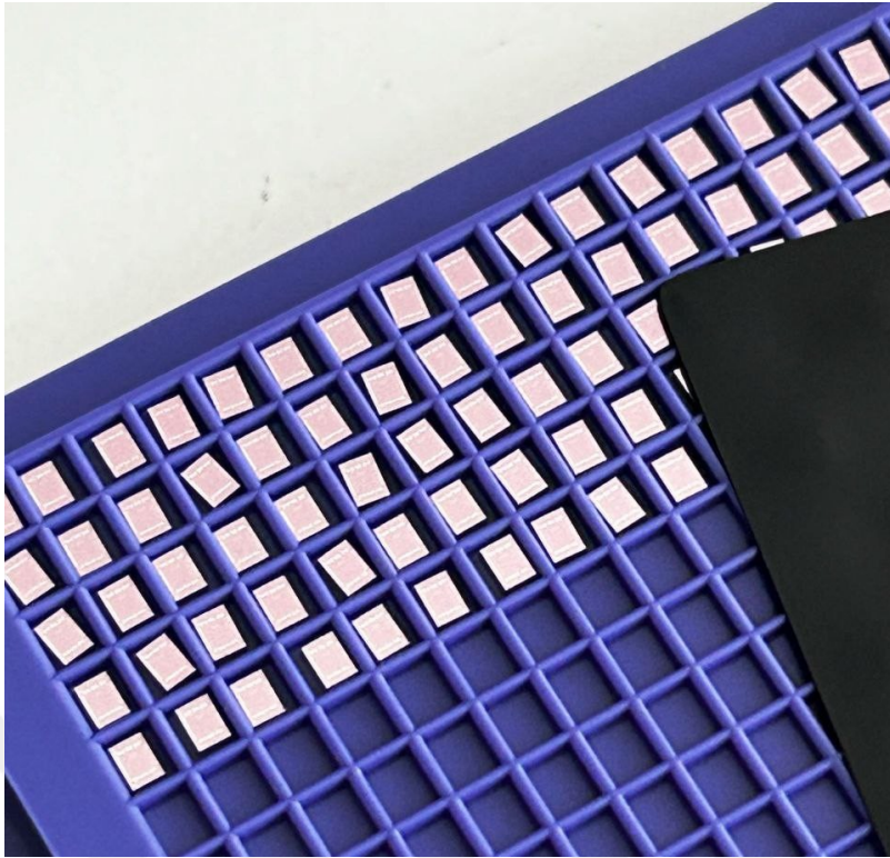
Figure 4.23 : Produced IC with the active shield digital design.
