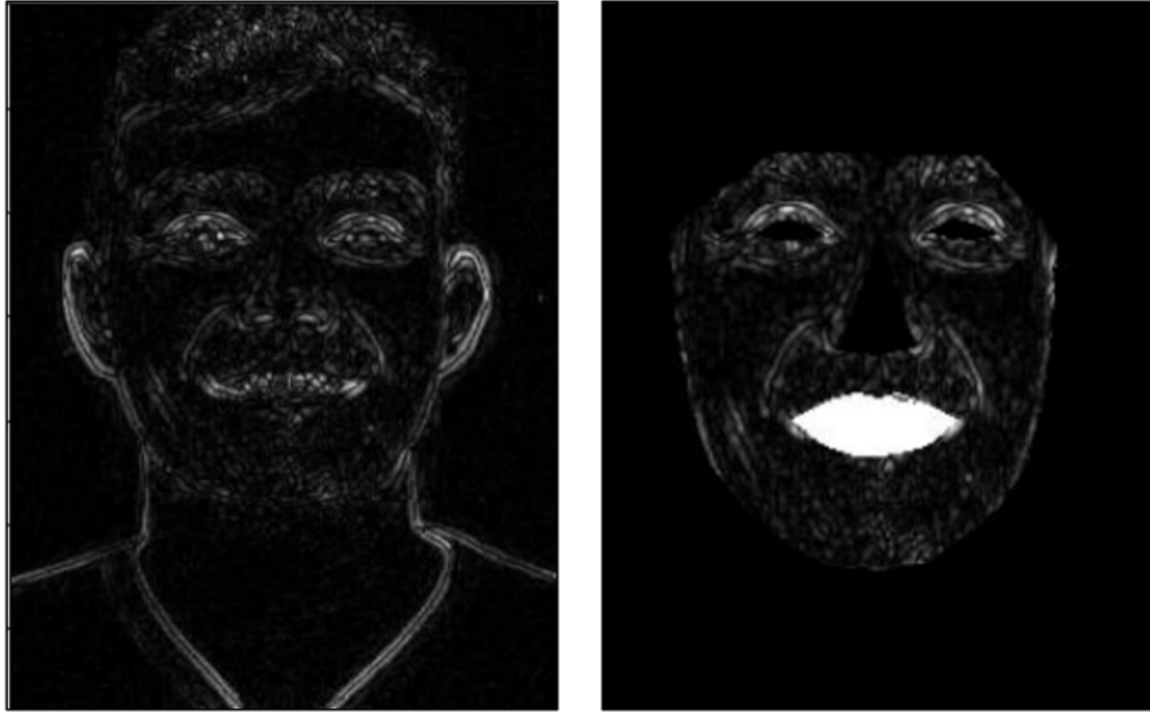
Figure 13. Texture part of the reference image (left), the filtered redundant parts and areas of the texture with a white-masked mouth, black-masked eyes, and black-masked nose (right)
