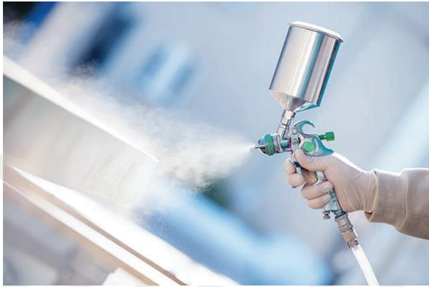
Figure 2.9. Spraying Application of Painting
