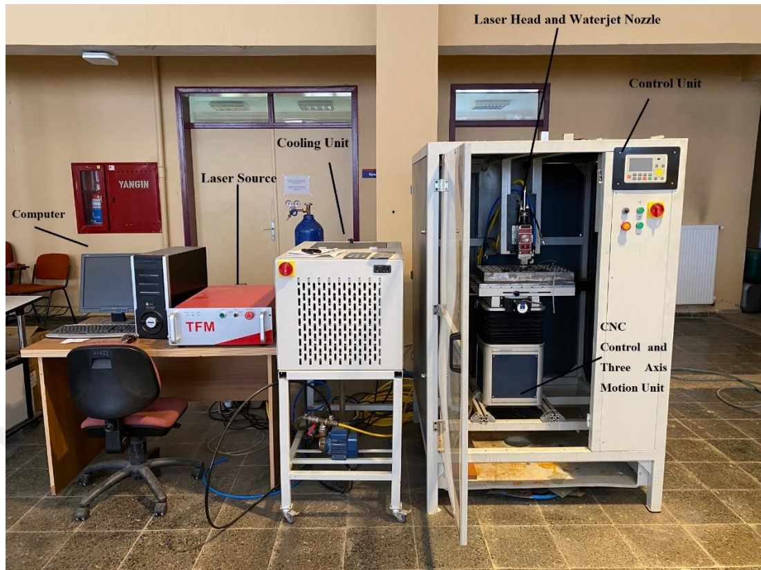
Figure 5.22 Assembly of waterjet guided laser system
