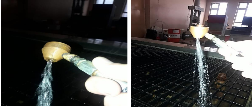
Figure 5.7 Water flow in one side inlet design
