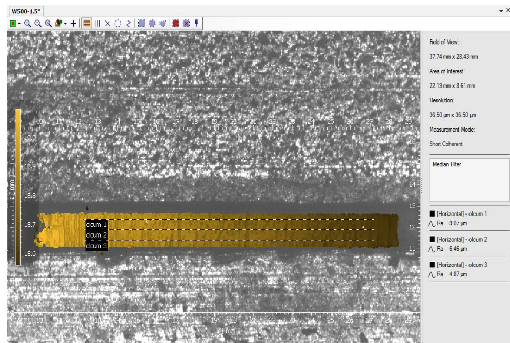
Figure 4.4 Roughness measurement method
