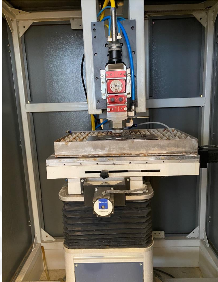
Figure 5.1 Experimental cutting design of waterjet guided laser cutting system
