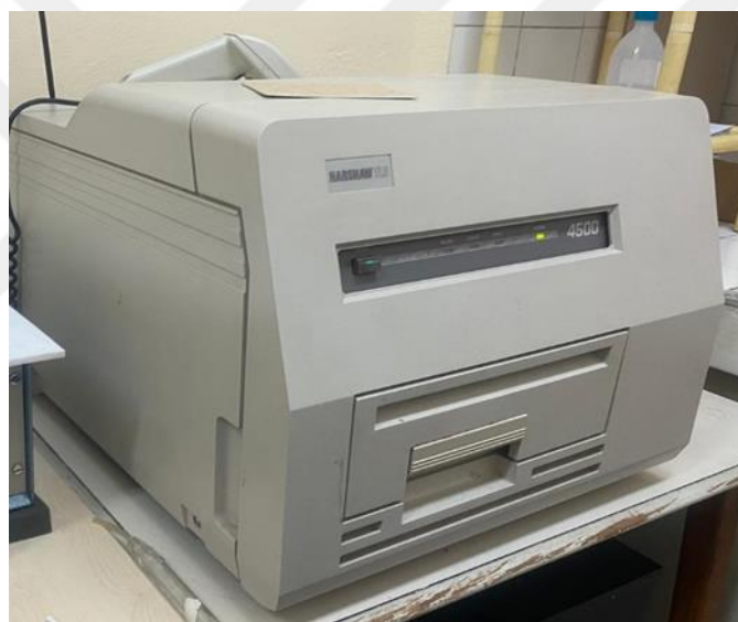
Figure 19 TLD reader, Harshaw 4500
