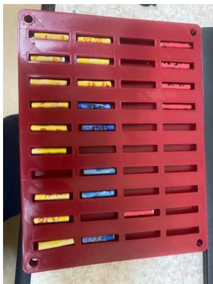
Figure 18 There are two TLDs in each of the yellow, blue and red tags.
